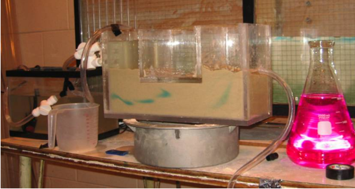
Figure 20. Dye tracing in the pore-water flow tank.
