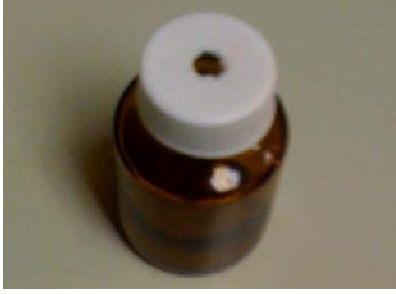
Figure 24. The container with a breach hole ( d_b = 0.56 cm) used as an experimental breached munition surrogate.
