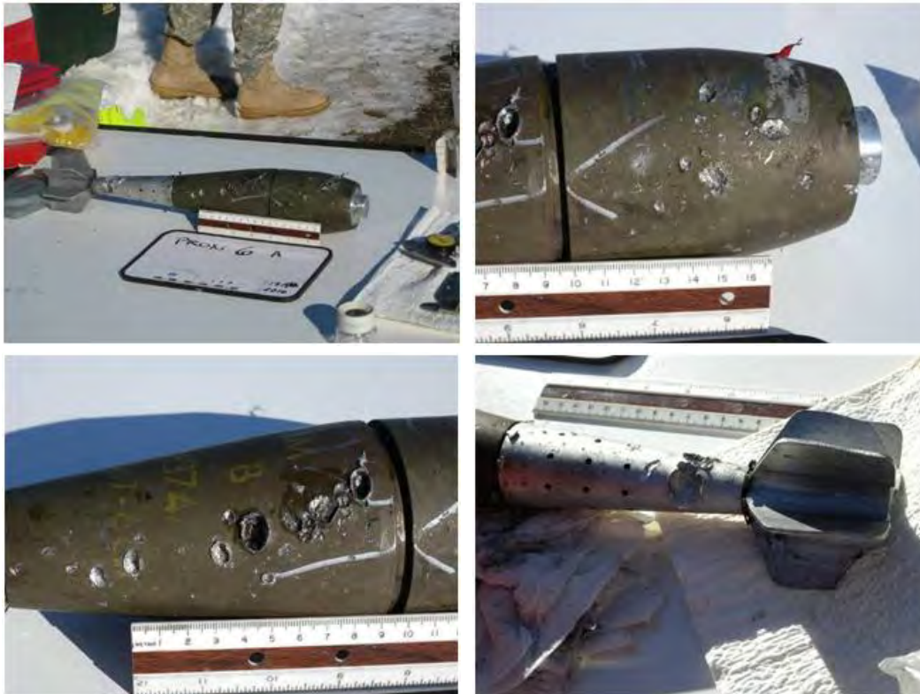
Figure 7-23. Damages recorded for test 6, round 6b (vertical incoming round, 0.50-m distance).
