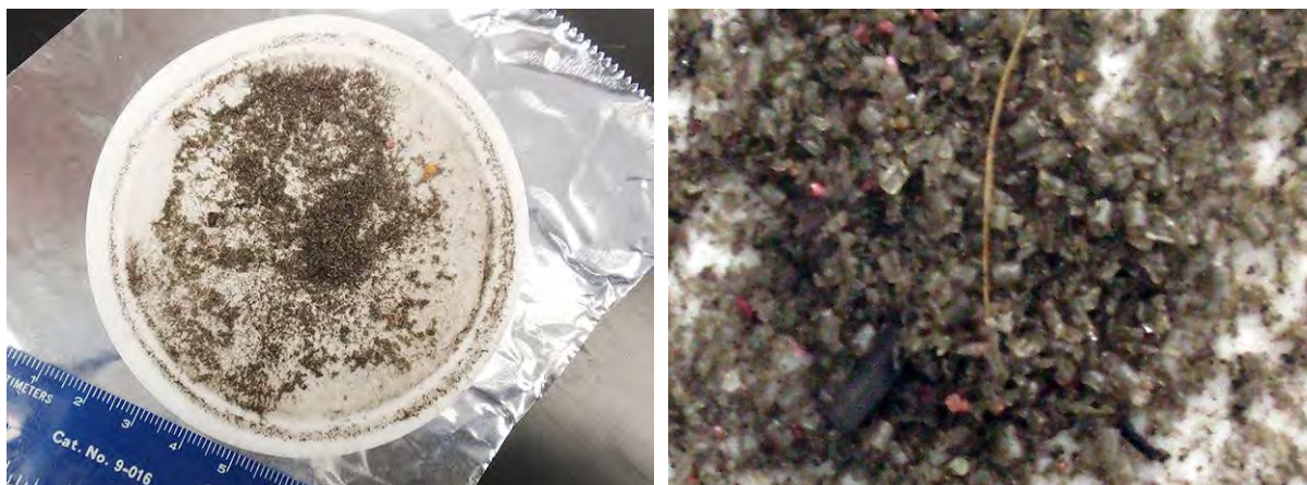
c. M2 propellant on filter.
