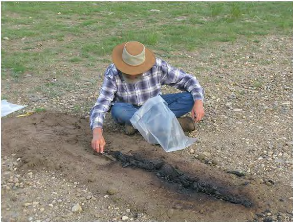
Figure 3-21. Sampling test pads following burning of propellants.
