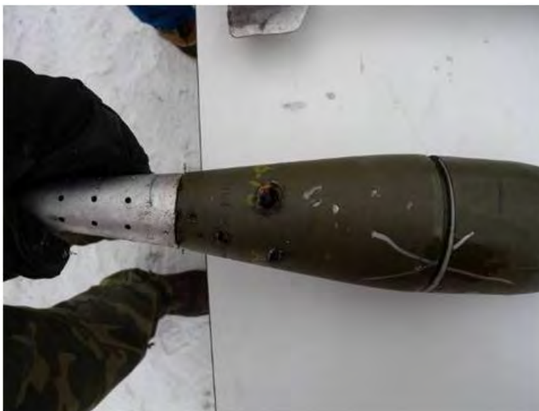
Figure 7-31. Damages recorded for test 11, round 11d (vertical incoming round, 1.00-m distance).
