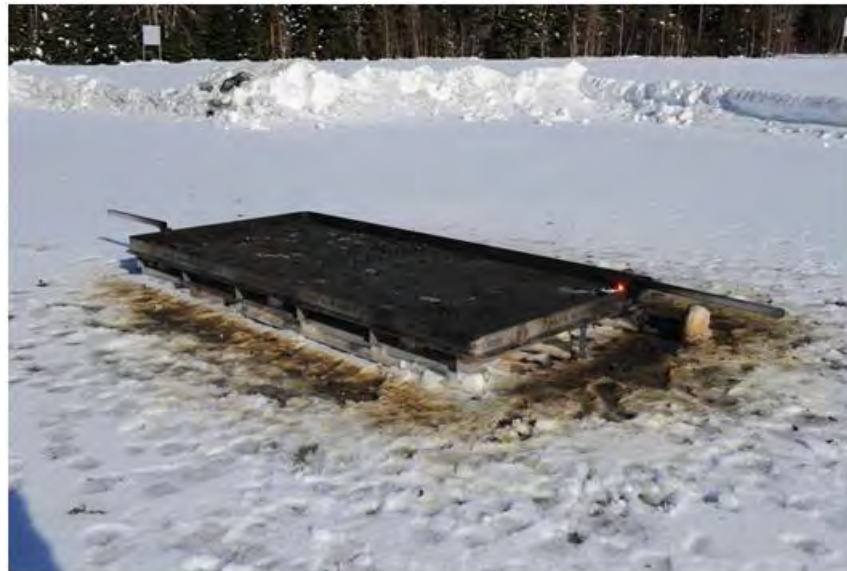
Figure 4-31. Residues projected outside the table, trial 3.
