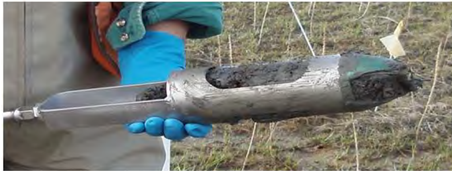
b. Stainless steel bucket auger equipped with a mud bit.
