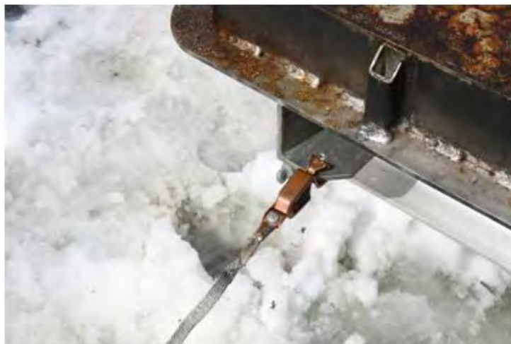
Figure 4-23. Grip to hold the conductive strap to the table.
