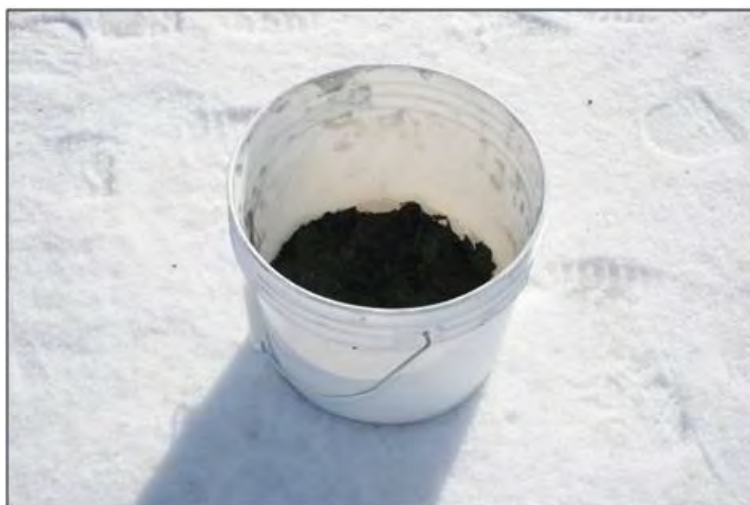
Figure 4-33. Burning residues from trial 3.
