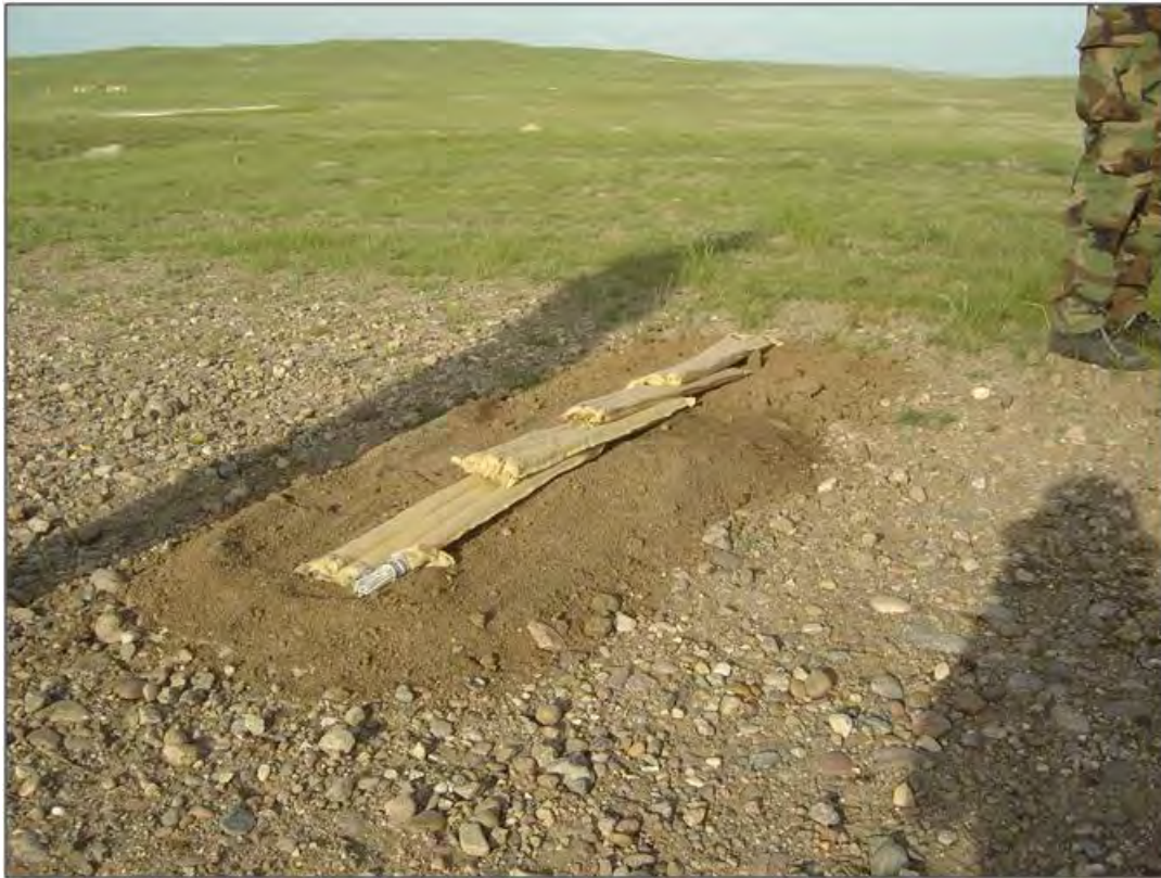
Figure 3-18. Setup of four charge 7 propellant bags on sand.
