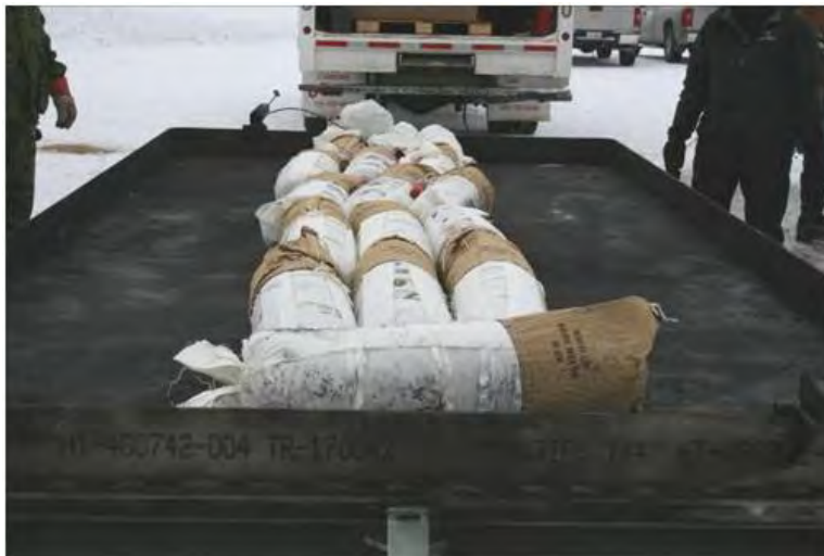
Figure 4-16. Prior to burning with 104 kg of M4 propellant load.
