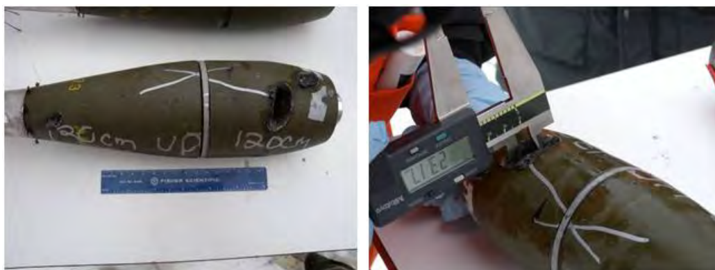
Figure 7-32. Damages recorded for test 11, round 11e (vertical incoming round, 1.20-m distance).
