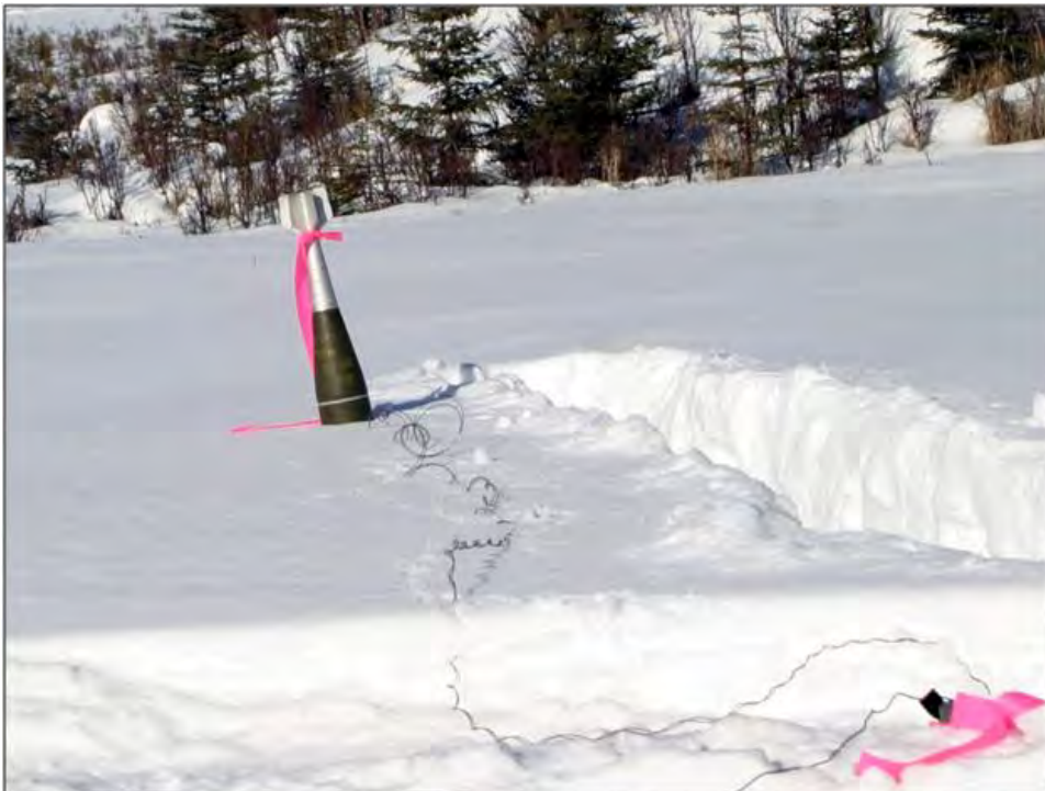
b. Round in place ready for detonation.
