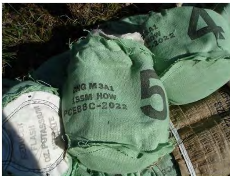
Figure 4-8. Bags of 155-mm charge 4 and 5 and the flash reducer pad
