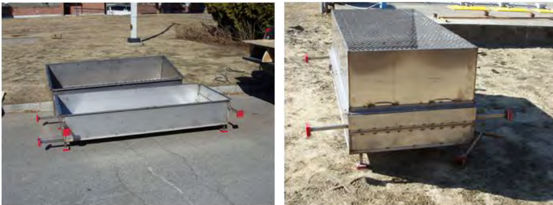
a. Pan (foreground) with bonnet removed.
