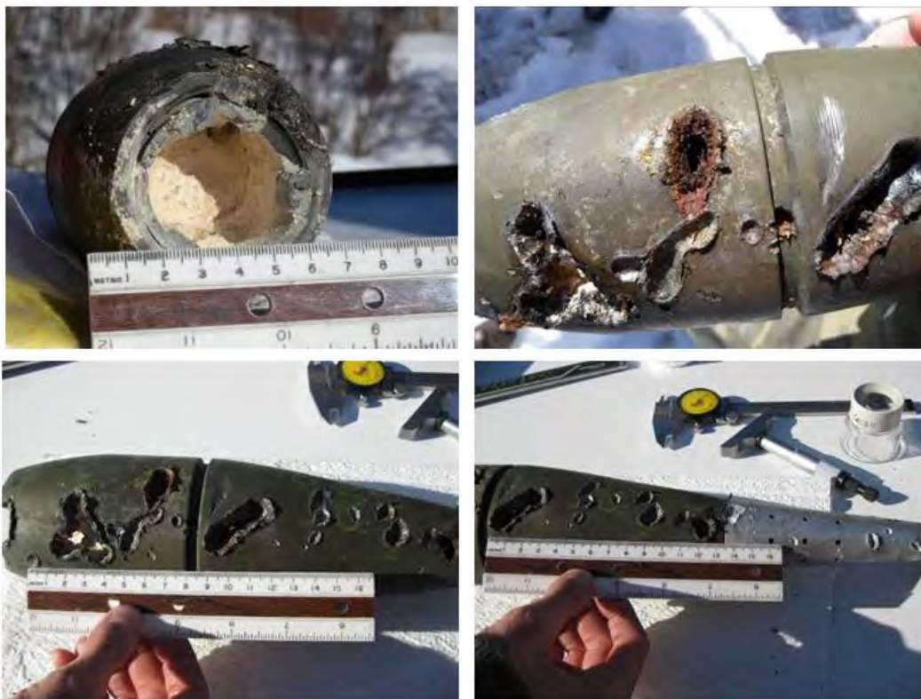
Figure 7-19. Damages recorded for test 3, round 3a (vertical incoming round, 0.50-m distance).
