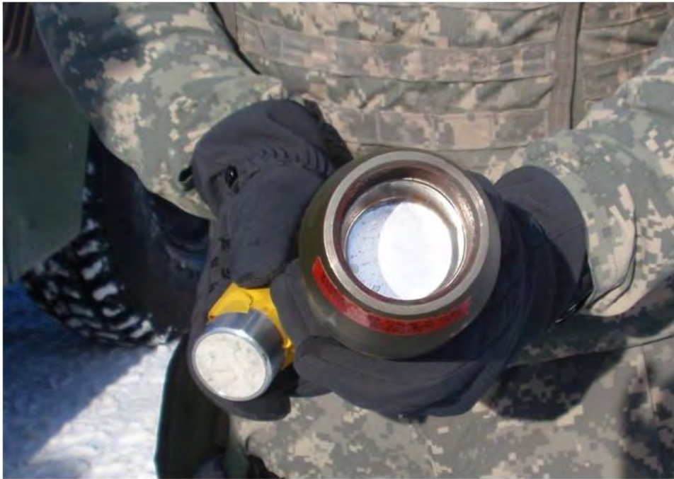
a. Preparing to screw the device into the 81-mm HE body.
