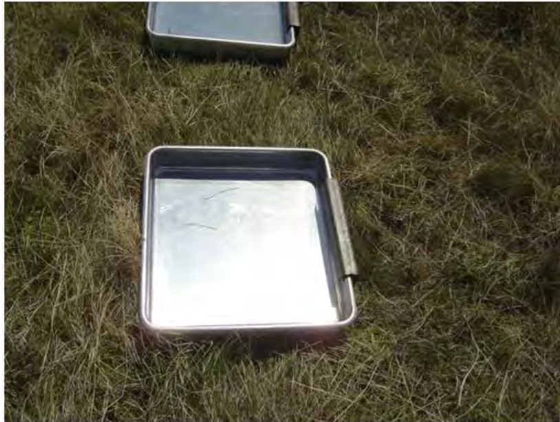
Figure 3-13. Particles trap in holder.
