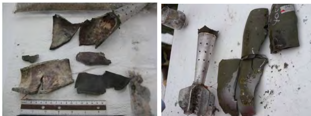
Figure 7-11. Typical 81-mm mortar metal pieces obtained after a partial detonation of a simulated UXO.
