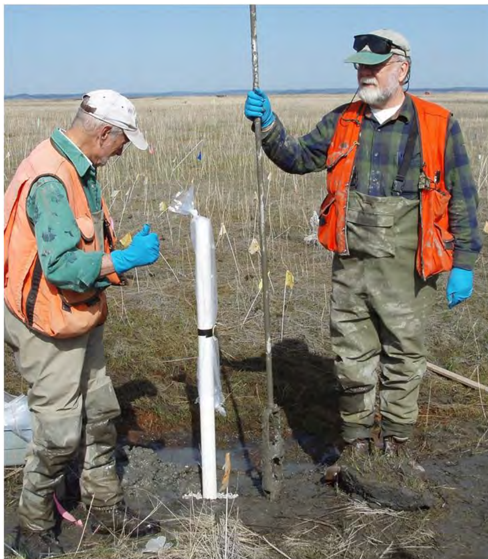
d. Finished well near the crater at L03 (14 May 2009). The vented protective PVC cap was installed during the next site visit.
