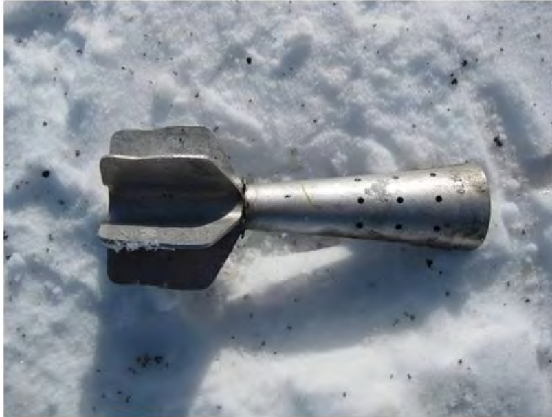
Figure 7-34. Tail recovered after sympathetic detonation of a UXO in test 9, round 9b (horizontal incoming round, 0.50-m distance).
