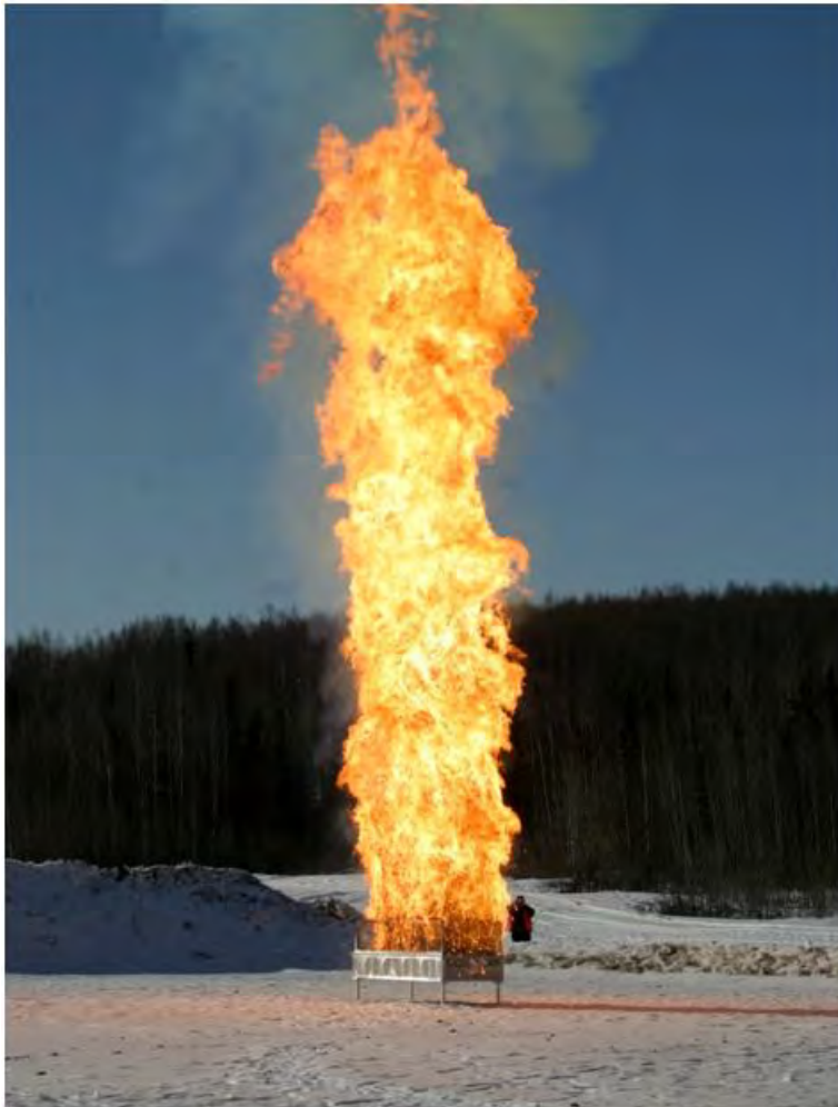
Figure 12-1. Propellant burn test, FP Neibar, Ft. Richardson, AK, March 2011.
