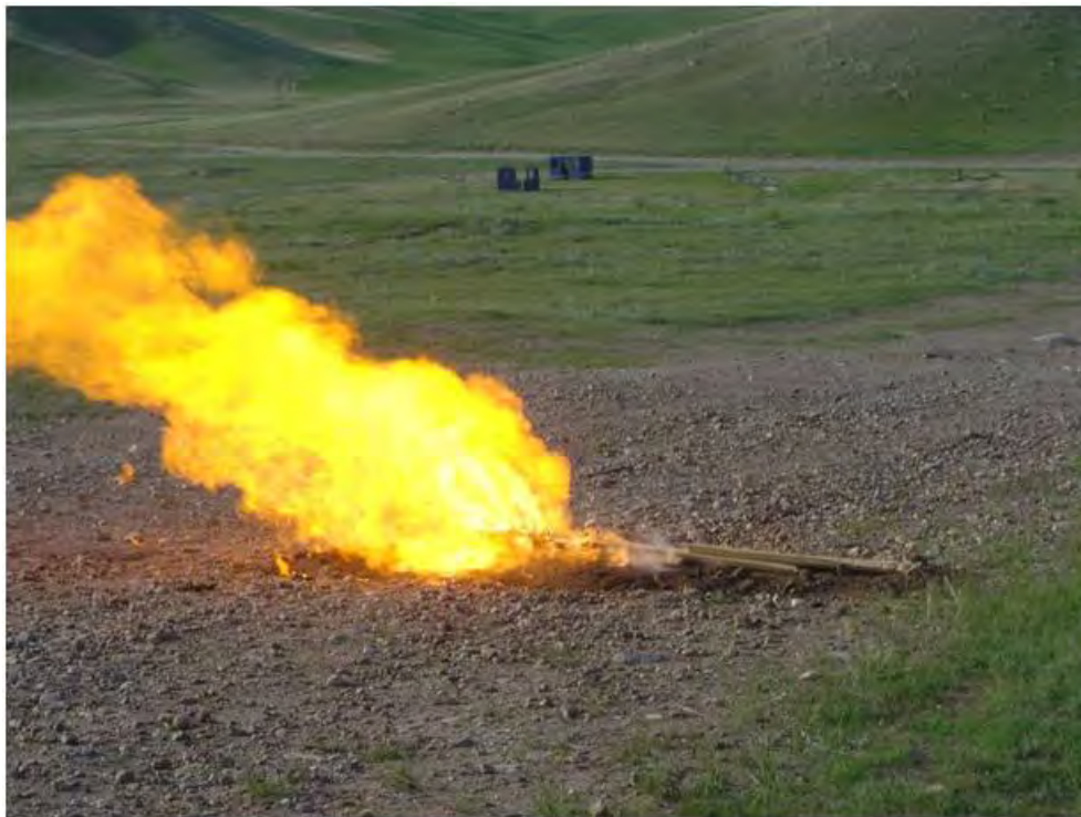
Figure 3-19. Ignition of four charge 7 propellant bags on sand.
