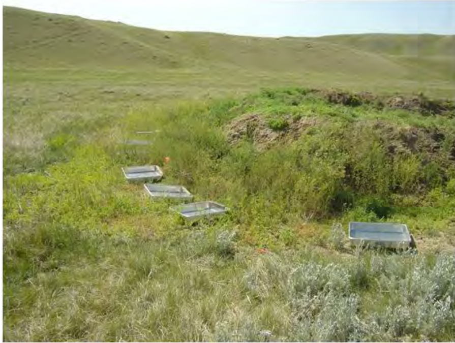
Figure 3-12. Gunside particles traps.
