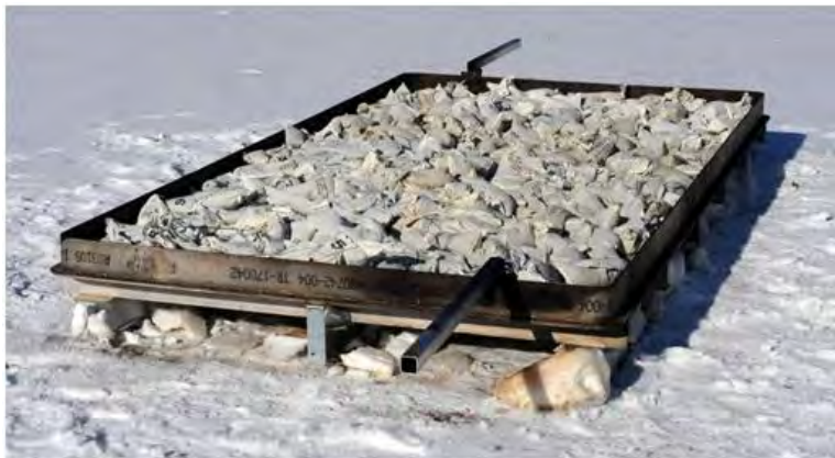
Figure 4-14. Prior to burning with 150 kg of M67 propellant load.
