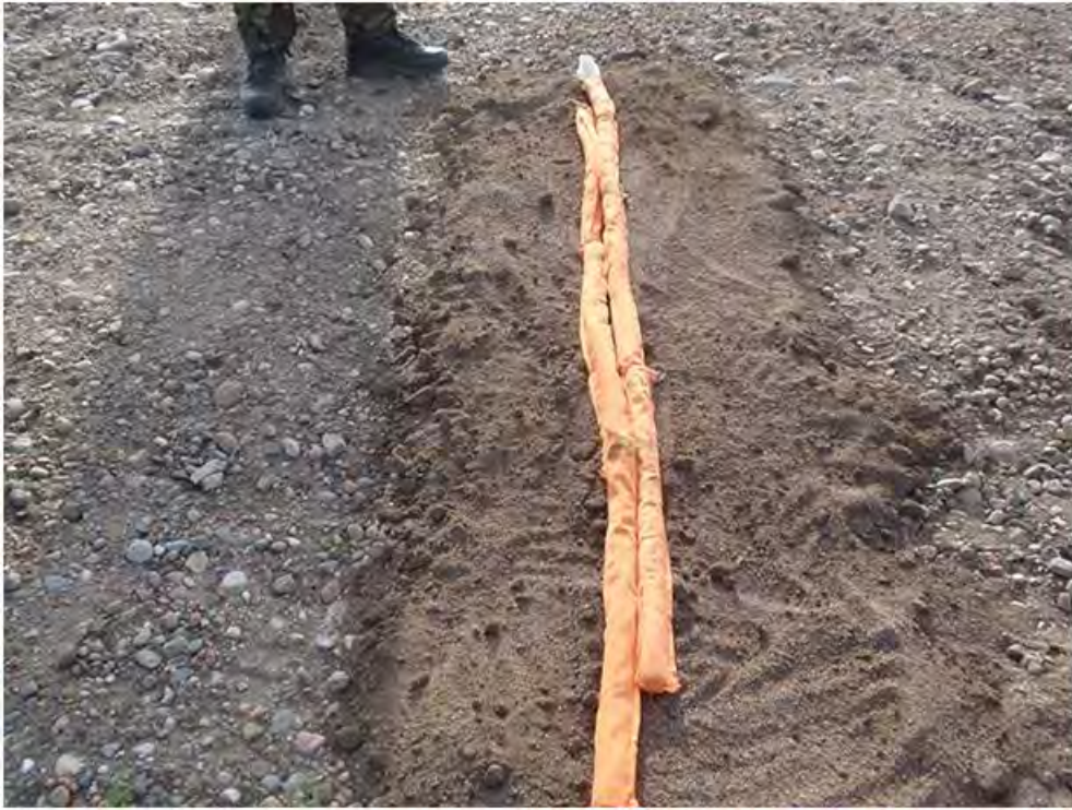
Figure 3-20. Setup of six charge 4 propellant bags on sand.
