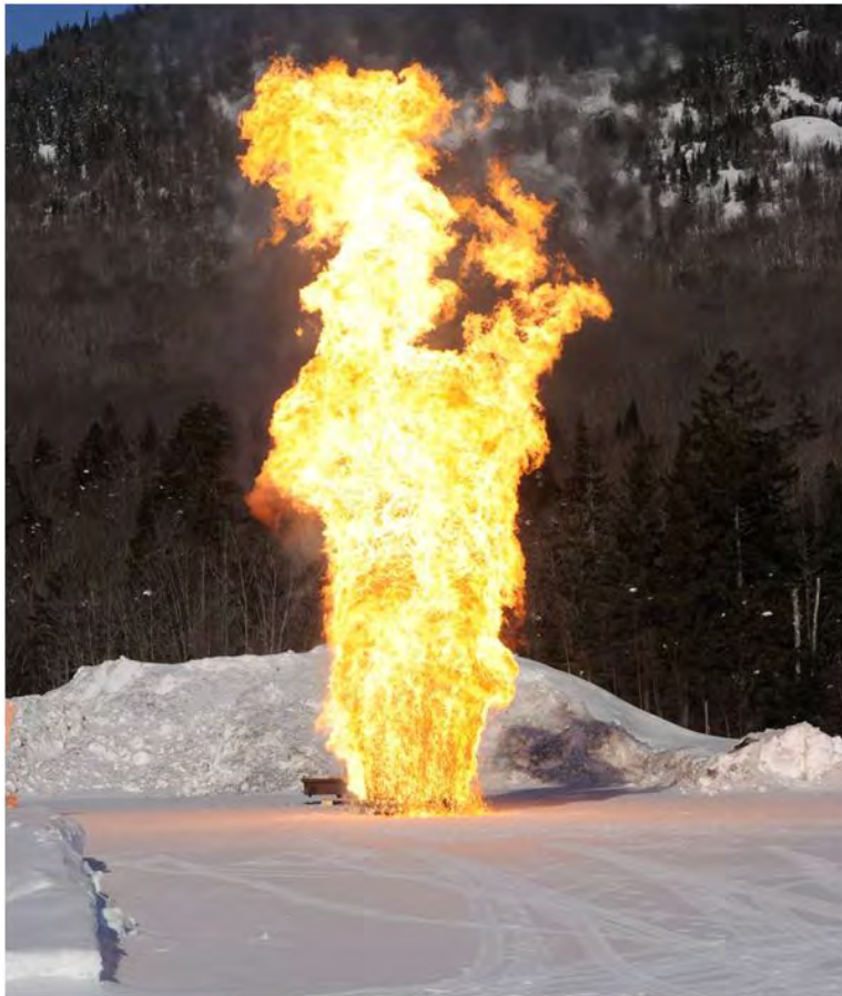
Figure 4-29. Maximum intensity of burning 10 s after ignition.
