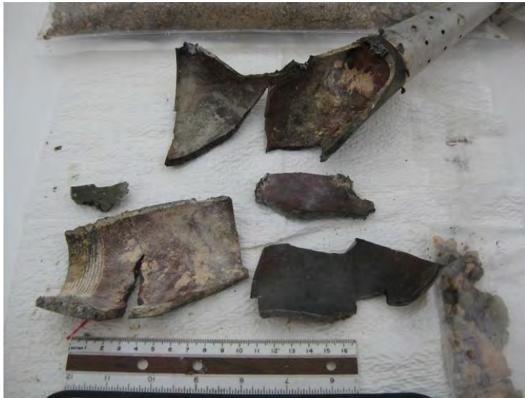
Figure 7-35. Damages recorded for test 10, round 10a (horizontal incoming round, 0.50-m distance).
