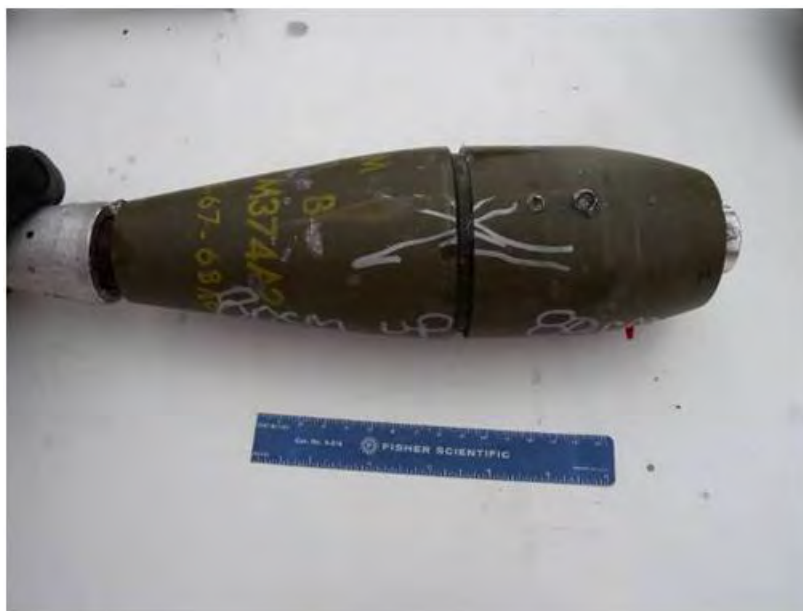
Figure 7-30. Damages recorded for test 11, round 11c (vertical incoming round, 0.80-m distance).
