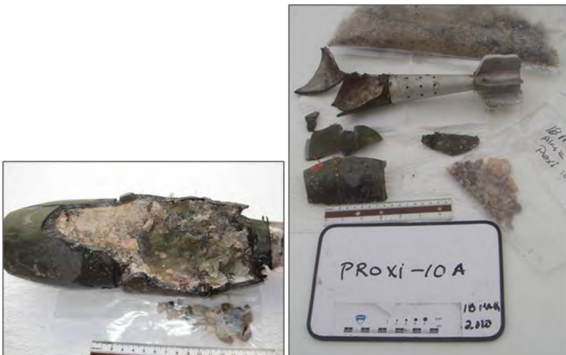
Figure 8-8. Residues recovered from round 9a (left) and round 10a.
