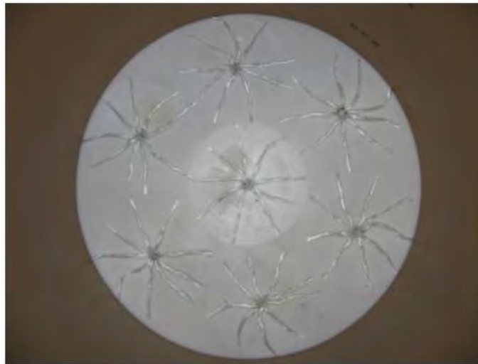
Figure 5-1. Fiberglass wicks positioned on the bottom of each column.
