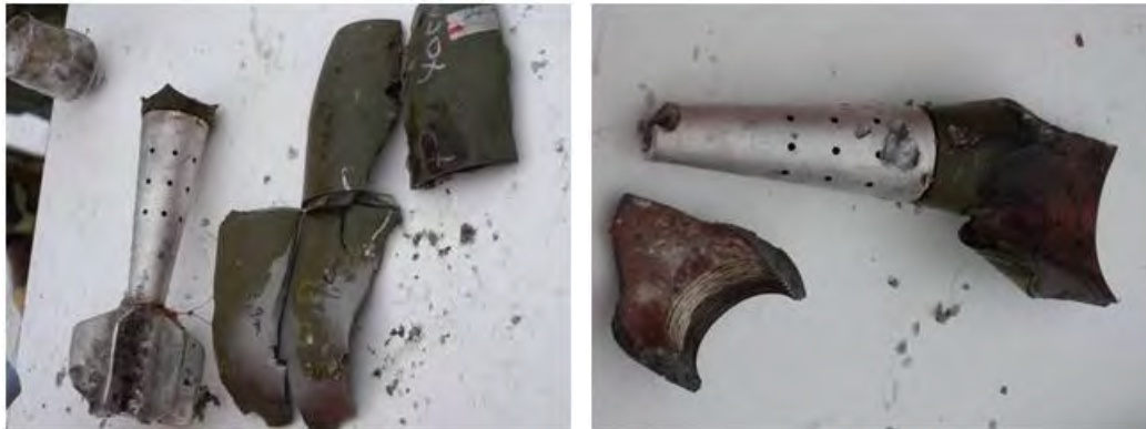
Figure 7-16. Damages recorded for test 11, round 11a (vertical incoming round, 0.40-m distance).
