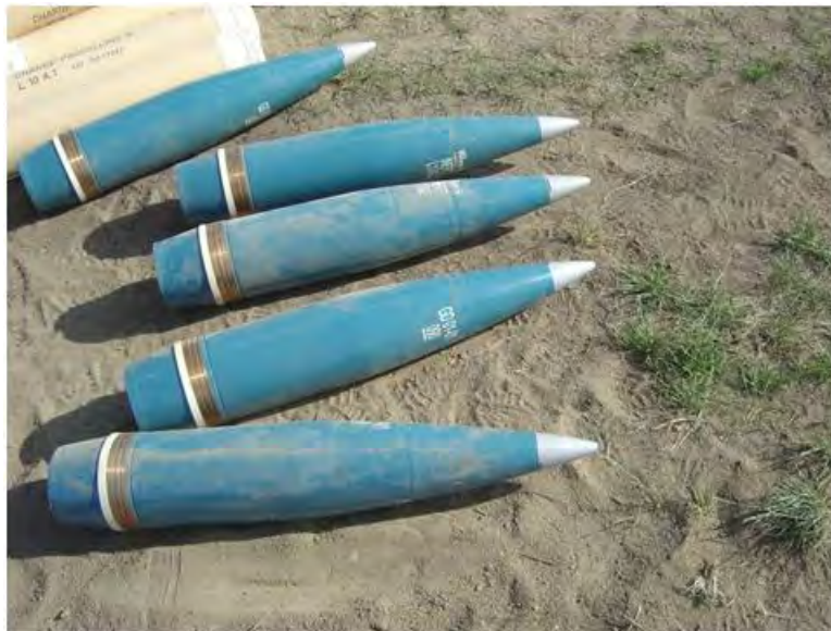
Figure 3-4. Shell of the 155-mm Practice Inert L17.
