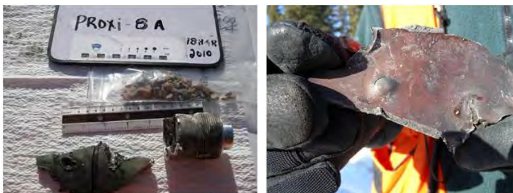
Figure 7-27. Damages recorded for test 8, round 8a (vertical incoming round, 0.50-m distance).
