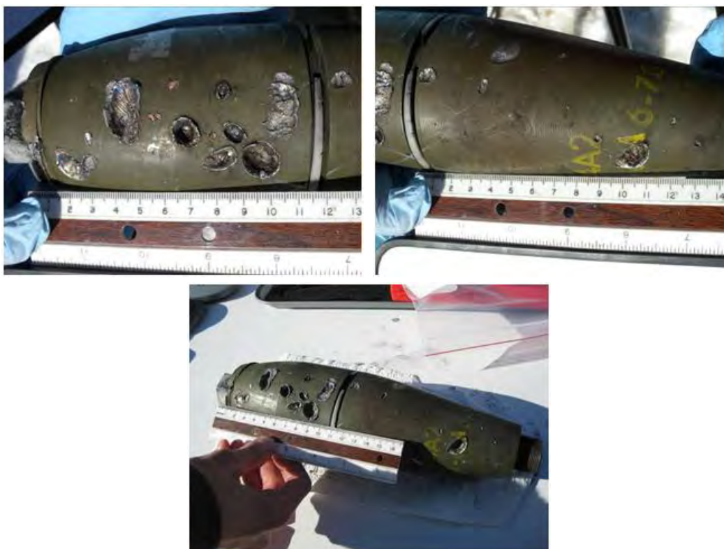
Figure 7-20. Damages recorded for test 3, round 3b (vertical incoming round, 0.50-m distance).
