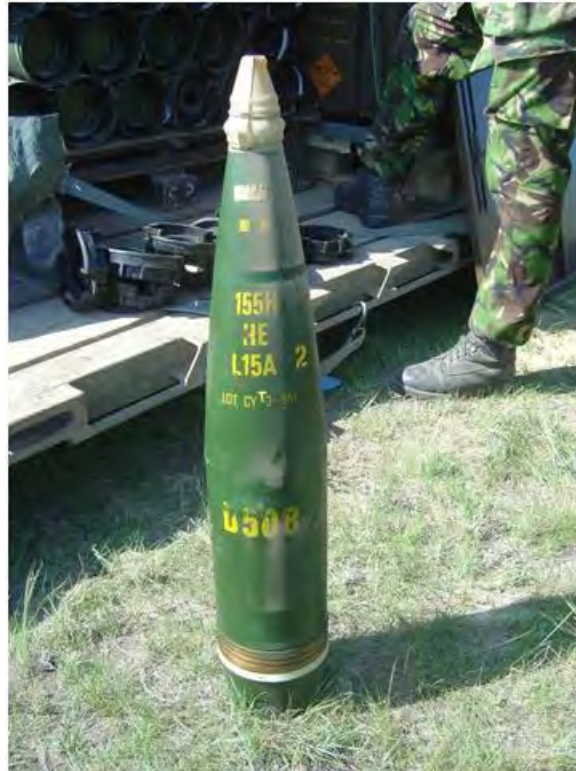
Figure 3-3. Shell of the 155-mm HE L15.
