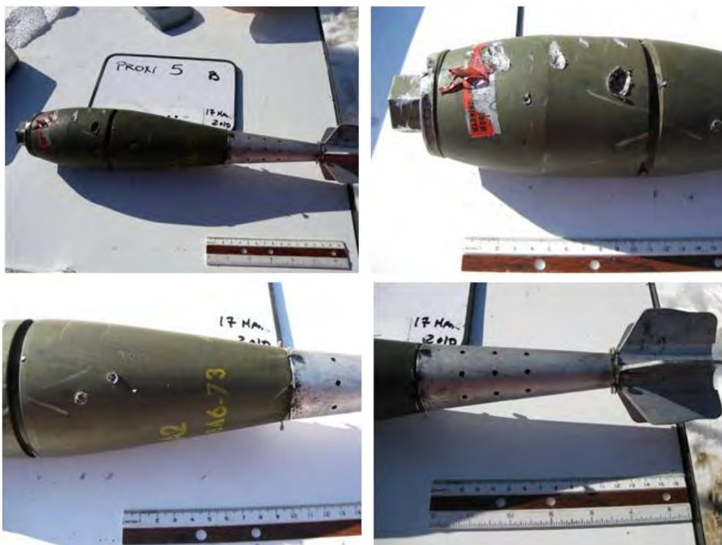
Figure 7-22. Damages recorded for test 5, round 5b (vertical incoming round, 0.50-m distance).
