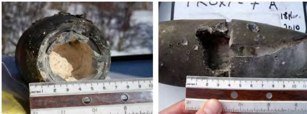
Figure 7-10. Typical breaches/cracks to an 81-mm mortar (simulated UXO).
