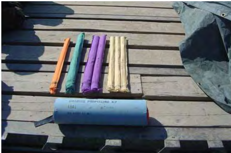
Figure 3-5. Propellant charge L8 A1.
