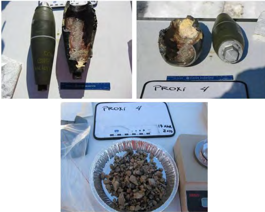
Figure 7-15. Damage recorded and HE chunks collected in test 4, round 4b (vertical incoming round, 0.30-m distance).
