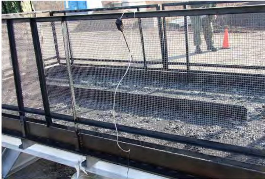
Figure 4-39. Thermocouples in the flame and 5 m away (orange cone) for radiation measurement.
