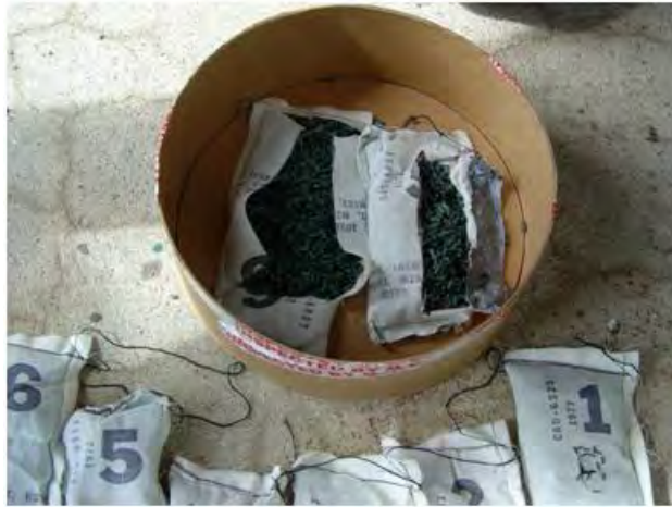
Figure 4-7. M1 propellant grains in bags 6 and 7.
