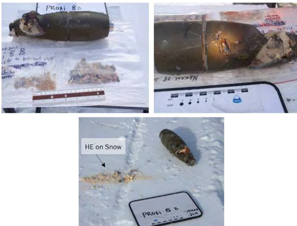
Figure 7-28. Damages recorded for test 8, round 8b (vertical incoming round, 0.50-m distance).
