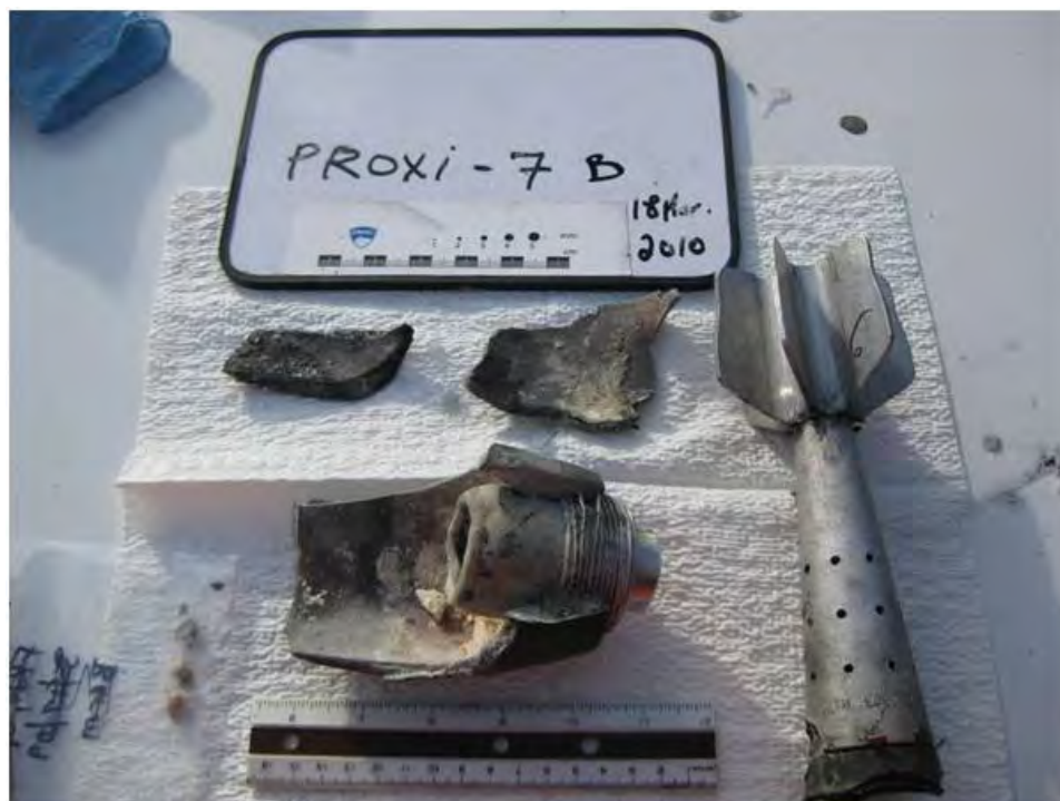
Figure 7-26. Damages recorded for test 7, round 7b (vertical incoming round, 0.50-m distance).
