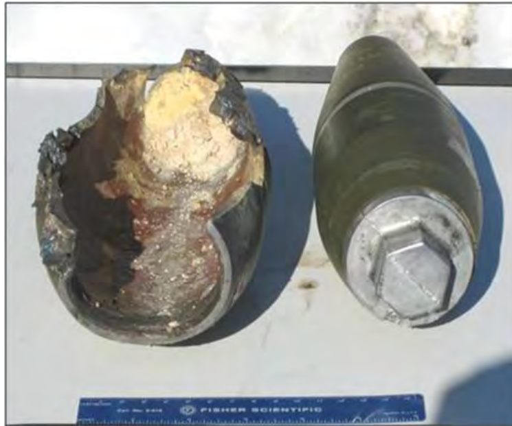
Figure 8-2. Cross-section of round 4b next to an undetonated 81-mm mortar projectile.
