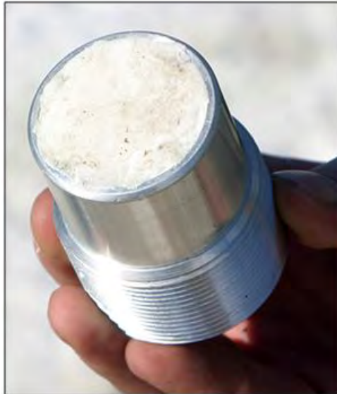
Figure 6-1. Device with C4 booster installed.
