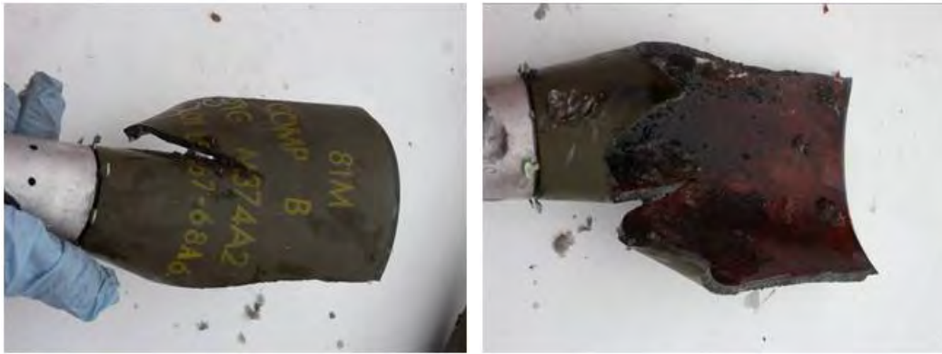
Figure 7-29. Damages recorded for test 11, round 11b (vertical incoming round, 0.60-m distance).
