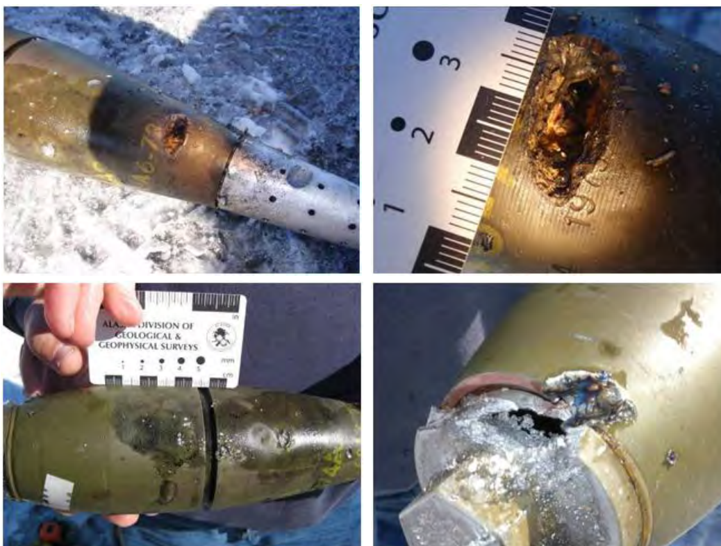
Figure 7-17. Damages recorded for the test1 round (vertical incoming round, 0.50-m distance).
