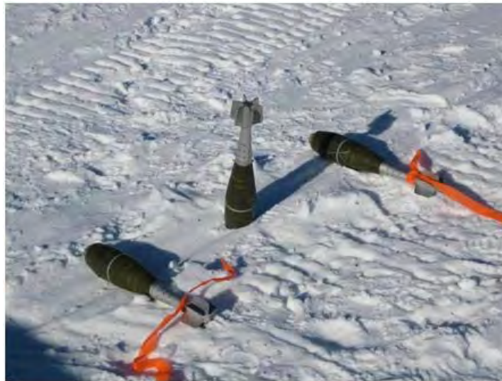
Figure 8-3. Setup used for test 4, with vertical “incoming” round to be set off high-order and two “UXO” placed 30 cm from the round.
