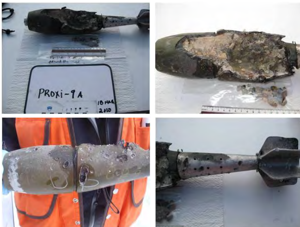
Figure 7-33. Damages recorded for test 9, round 9a (horizontal incoming round, 0.50-m distance).
