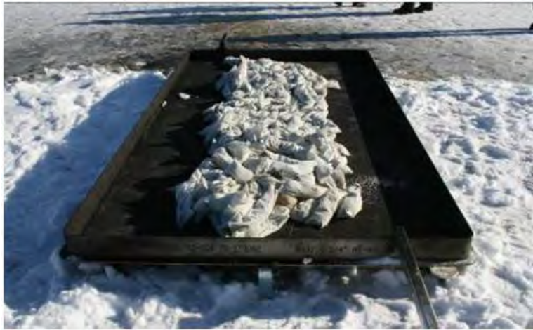
Figure 4-15. Prior to burning with 75 kg M67 propellant load.
