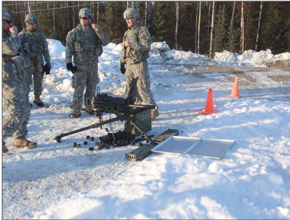
Figure 2-6. Location of trays used to collect propellant debris.
