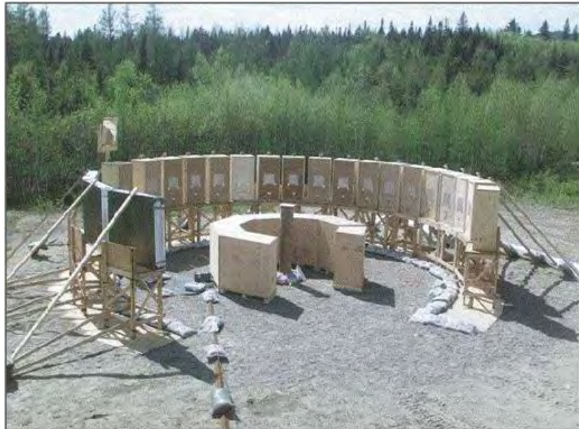
Figure 7-2. Typical setup for arena tests. The munition is placed in the center stand. (Photo courtesy of Claude Fortier, DRDC Valcartier.)
