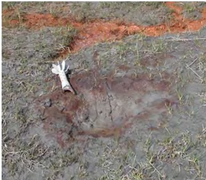
Figure 9-2. Image showing the crater at L03 in 2006. The red staining is from photo-transformation of TNT. A monitoring well was installed adjacent to the north edge of this crater in May 2009.
