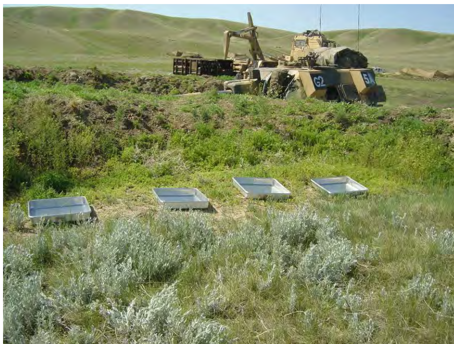
Figure 3-11. Particles traps beside the gun.
