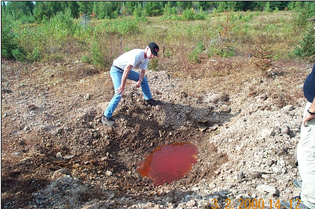
Figure 2-10. Reddish-colored crater formed from a low-order 500-lb bomb at CFB Gagetown.
