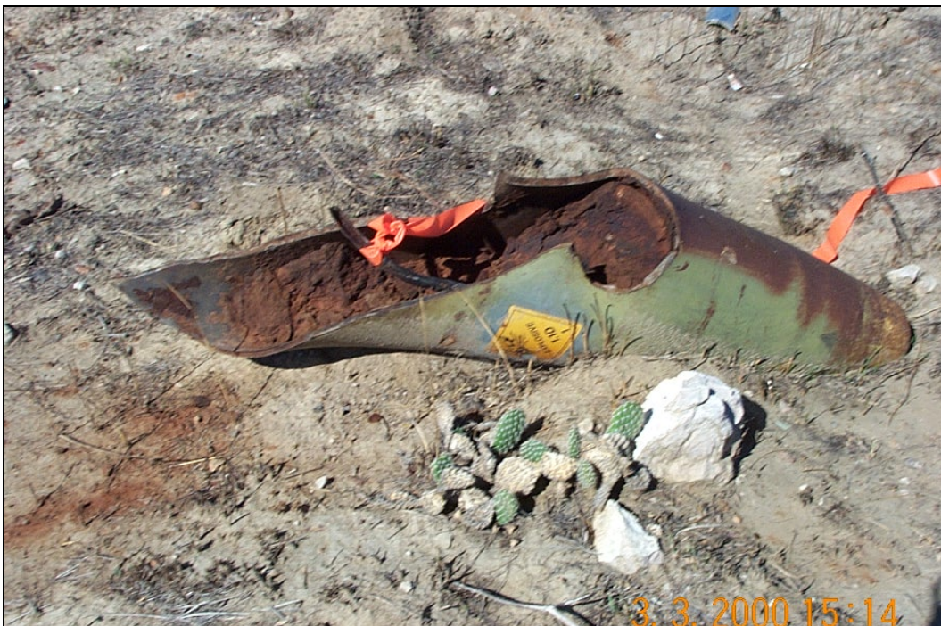
Figure 2-11. Low-order bomb found on the impact range at Camp Guernsey, WY.
