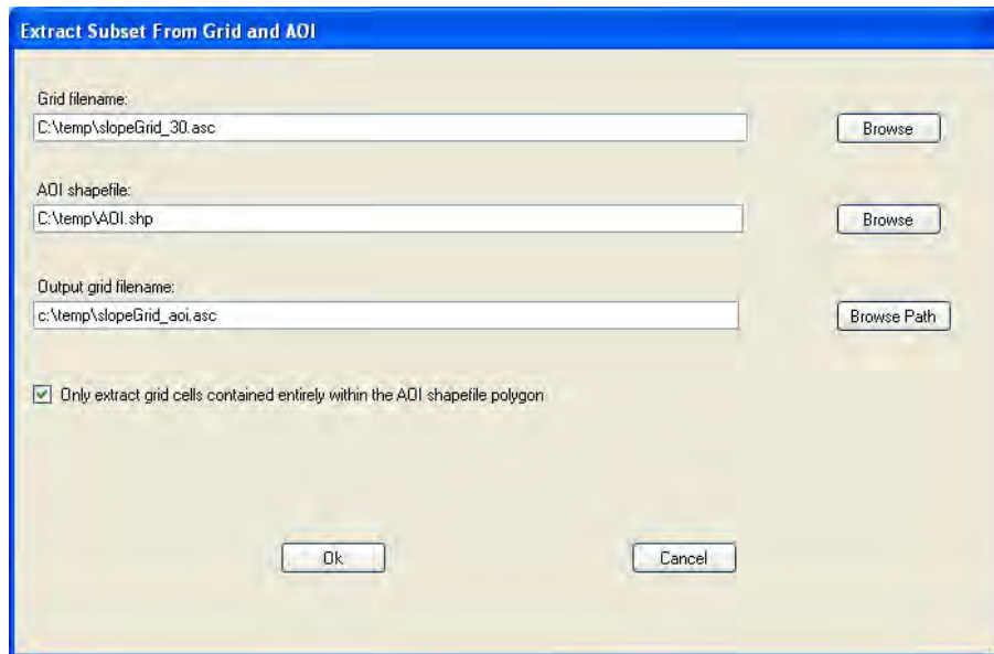
Figure A46. An example of the Extract Subset tool showing the inputs for creating a slope grid that coincides with the user’s AOI.
