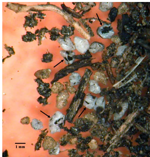
Fig. 3. Optical image showing TNT particles (arrows) in residue from a 'high-order' detonation. The TNT particles are opaque white to gray and often have black soot patches on parts of their surfaces.
