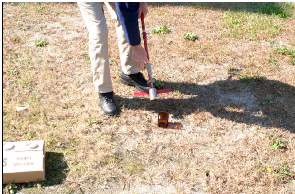
Figure 4. Coring tool (4.5-cm) used to collect discrete samples at Fort Hood, Texas.
