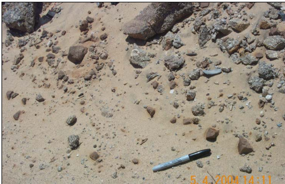
Figure 9. Small pieces of explosive observed on the surface of the soil at the Emerson Lake Range at 29 Palms, California.
