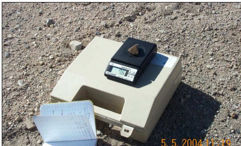
Figure 16. Field scale measuring the mass of a chunk of explosive found at Fort Hood, Texas.
