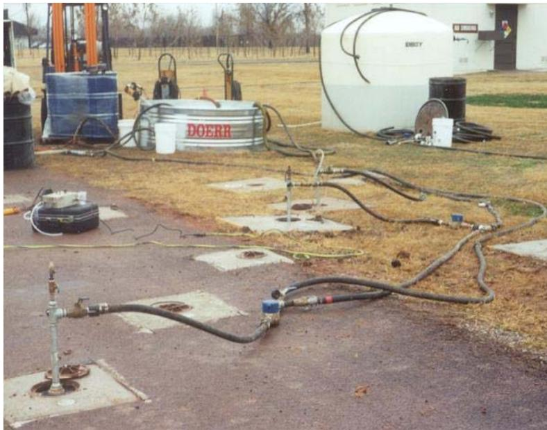
**Figure 3.11** Typical injection system layout showing injection wells, feed lines with flowmeters and control valves, injection pump, emulsion mixing tank, and makeup water tank.
