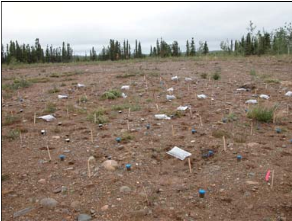
Figure 4. Grid (10-m x 10-m) at FP Mark where discrete and multi-increment samples were collected in July 2003.
