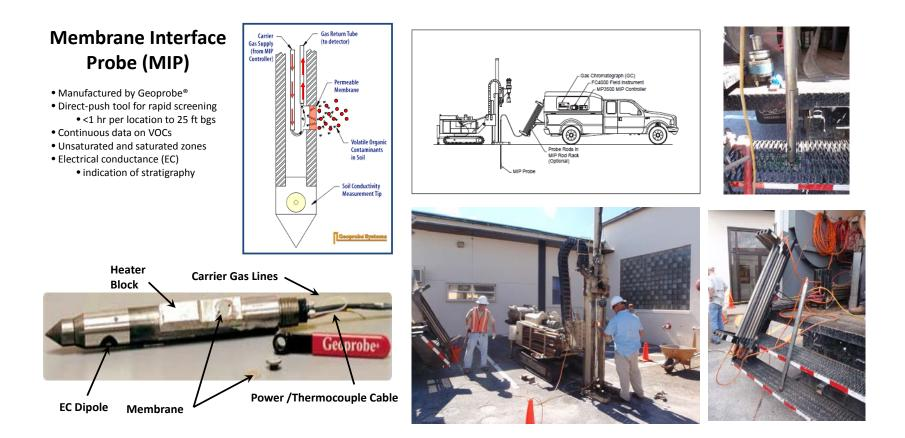
**Figure 5.4**. Schematic of Geoprobe MIP system, including use of the system during the ESTCP ER-201032 field demonstration (Source: Geoprobe SOP, 2012; http://geoprobe.com/literature/mip-logging-sop).
