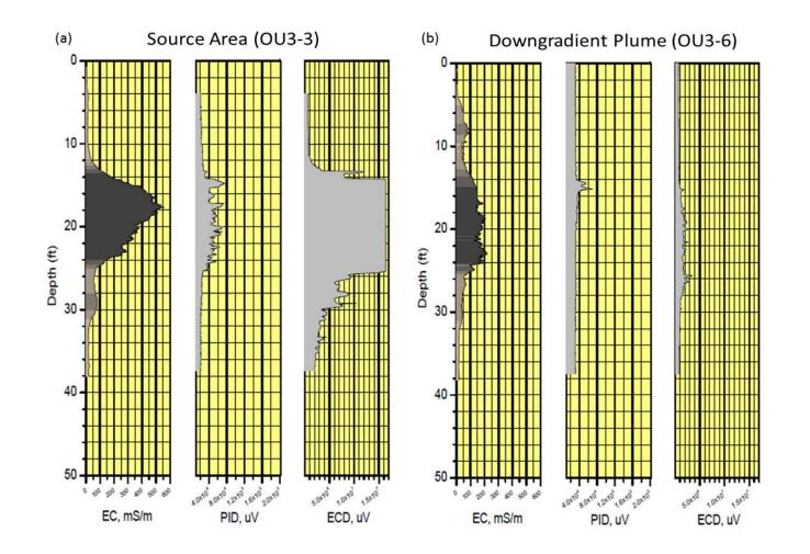
Figure 5.10. Example of MIP Dataplots along Plume Flowpath at Former Building 106 Source Area: (a) near source area, and (b) downgradient plume area.
