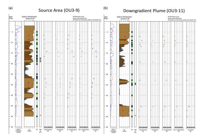
**Figure 5.12. Example of Waterloo** APS TM **Results at Building 780 Source Area:** (a) near source area, and (b) downgradient plume area showing the I<sub>k</sub>, groundwater VOC concentrations, along wth other complementary data collected including drive rate and potentiometric surface.
