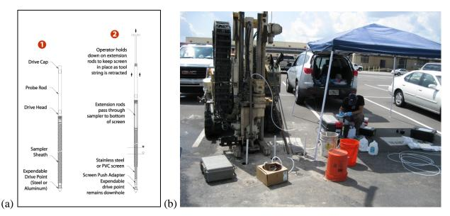
**Figure 5.8**. **Multi-Level Groundwater Sampling:** (a) Schematic of Geoprobe SP16 sampler operation (from <u>http://geoprobe.com/sp16-groundwater-sampler</u>); (b) Groundwater sampling during the ESTCP ER-201032 field demonstration, using Geoprobe SP16 system (via the direct-push rig) and temporary piezometers (installed in small diameter boreholes in foreground).
