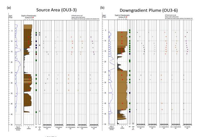
**Figure 5.11. Example of Waterloo** <sup>APS TM</sup> **Results at Two Locations at Former Building 106 Source Area:** (a) near source area, and (b) downgradient plume area showing the I<sub>k</sub>, groundwater VOC concentrations, along with other complementary data collected including drive rate and potentiometric surface.
