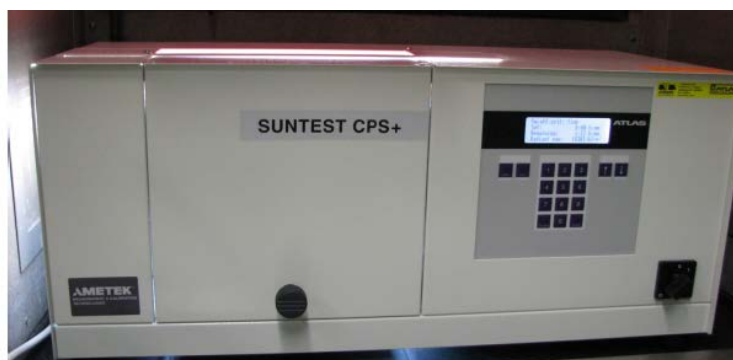
Figure 18. SUNTEST CPS+ Xenon Test Instrument used to evaluate phototransformation of NTO and DNAN in solution.
