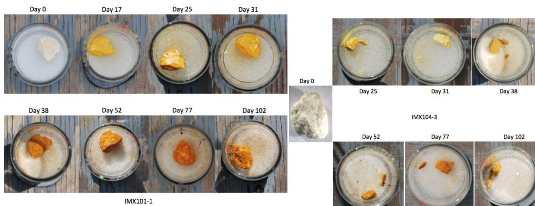
Figure 16. Sequential images of IMX101 particle #1 and IMX104 particle #3.
