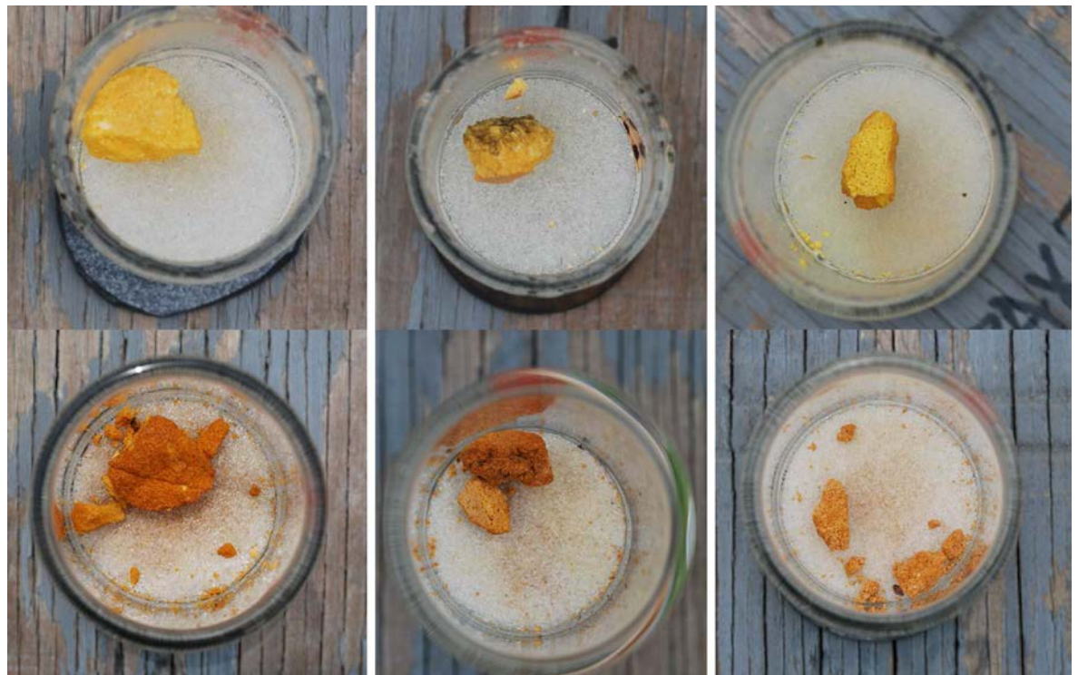
Effects of outdoor weathering and dissolution on three insensitive munitions formulations after 17 days (top) and 1 year (bottom).
