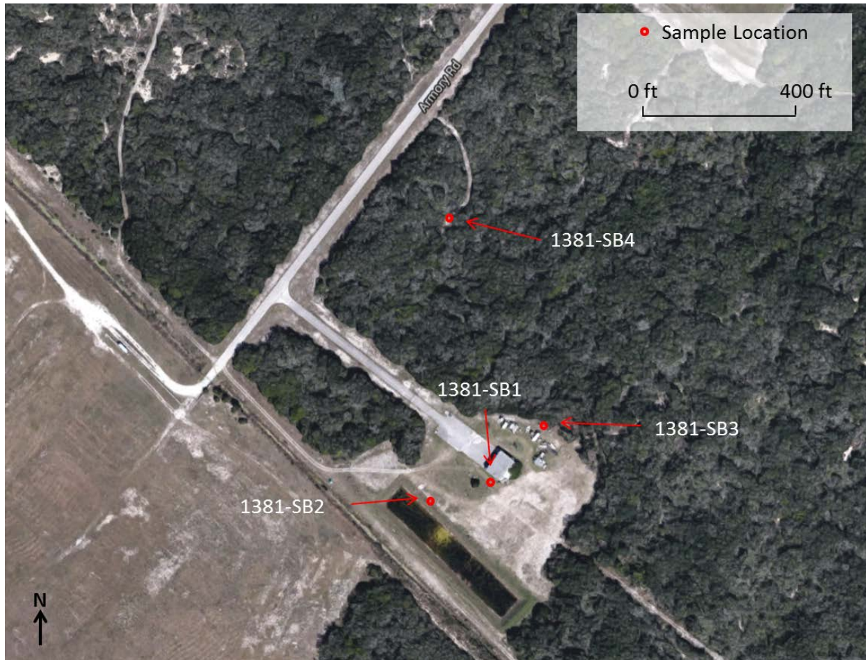
Figure 101. Locations for Investigation Points at Facility 1381, Cape Canaveral Air Force Station. At each location, vertical profiling, soil sub-sampling, and groundwater sampling was completed. Source area is in vicinity of location 1381-SB1. Groundwater flows in multiple directions from source area, including both northwest and southwest (toward canal and newly-installed interceptor trench).
