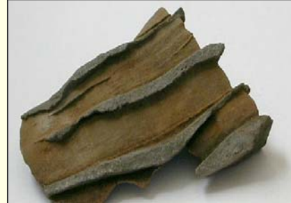
Interbedded transmissive (sandstone) and low permeability zones (shale).
