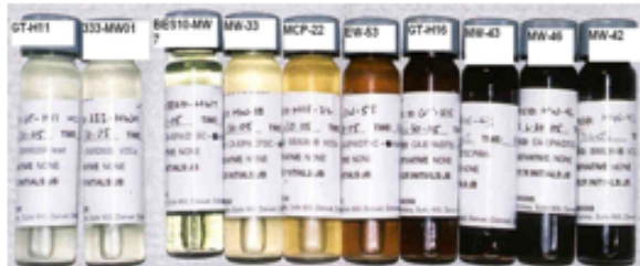
Various weathered LNAPL samples from ten monitoring wells across a single release site.
