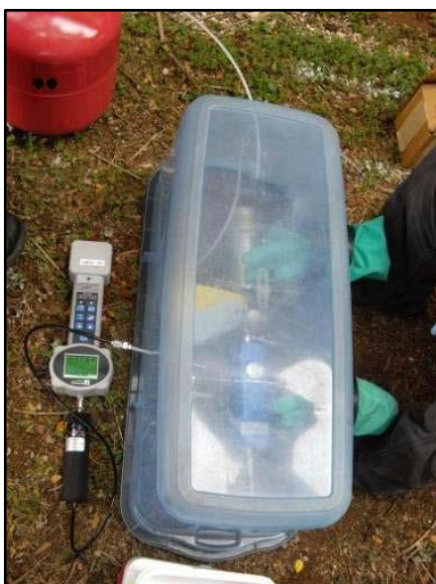
Figure D.3-6. Covering the entire sampling system & probe with a shroud. Reproduced from CRC CARE (2013).
