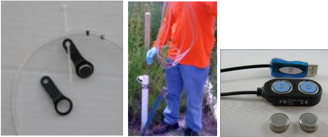
Figure G.2-4. Use of existing monitoring well and dedicated temperature logger string for approximation of the adjacent soil temperature profile. Courtesy of Ririe & Sweeney (2016) and Maxim Integrated, ( www.maximintegrated.com )
