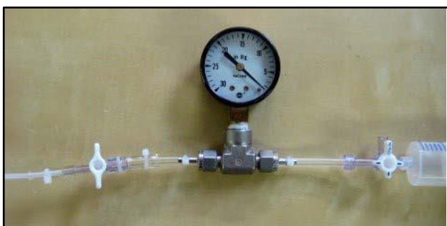
Figure D.3-5. Simple sampling train arrangement with vacuum gauge for a shut-in test. Reproduced from CRC CARE (2013).
