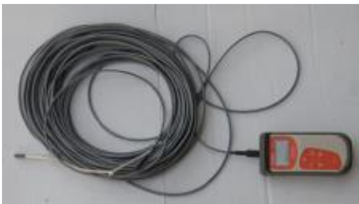
Figure G.2-3. Thermocouple reel to measure adjacent soil temperature profile. Courtesy of Ririe & Sweeney 2016)
