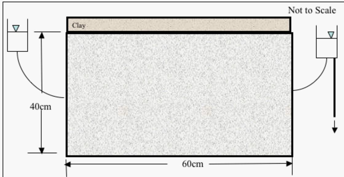
Figure 37 - Schematic of packing configurations of small tank – side view.
