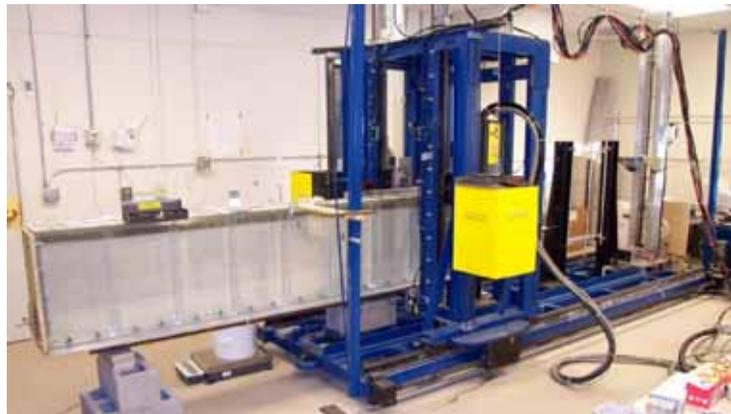
Figure 36 - Intermediate scale tank mounted on the x-ray platform.
