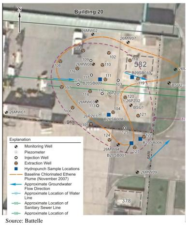
Figure 7-1. ISCO Target Treatment Area
