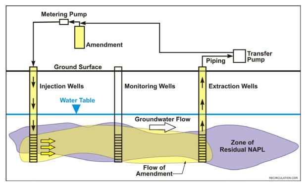
Figure 4-2. Typical Recirculation System
