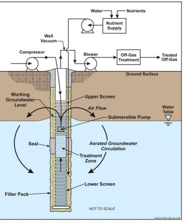
Figure 4-4. Conceptual Illustration of a Recirculation Well
