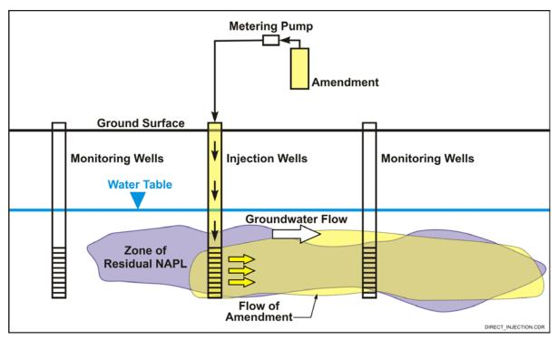
**Figure 4-1. Conceptual Illustration of a Direct Injection Process**
