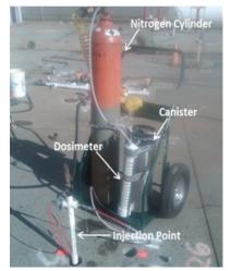
Source: Battelle Figure 7-4. Bioaugmentation Equipment
