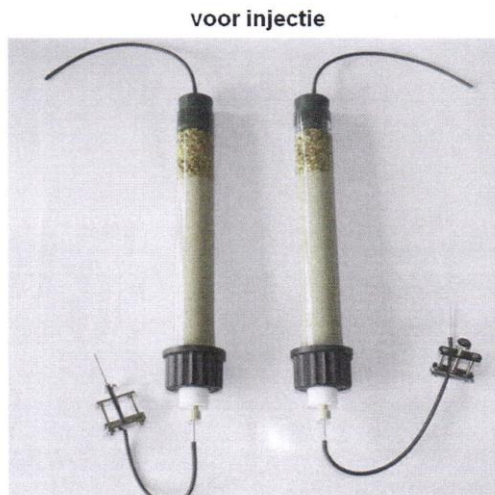
Photo 2 Tube test before and after injection of the iron slurry
