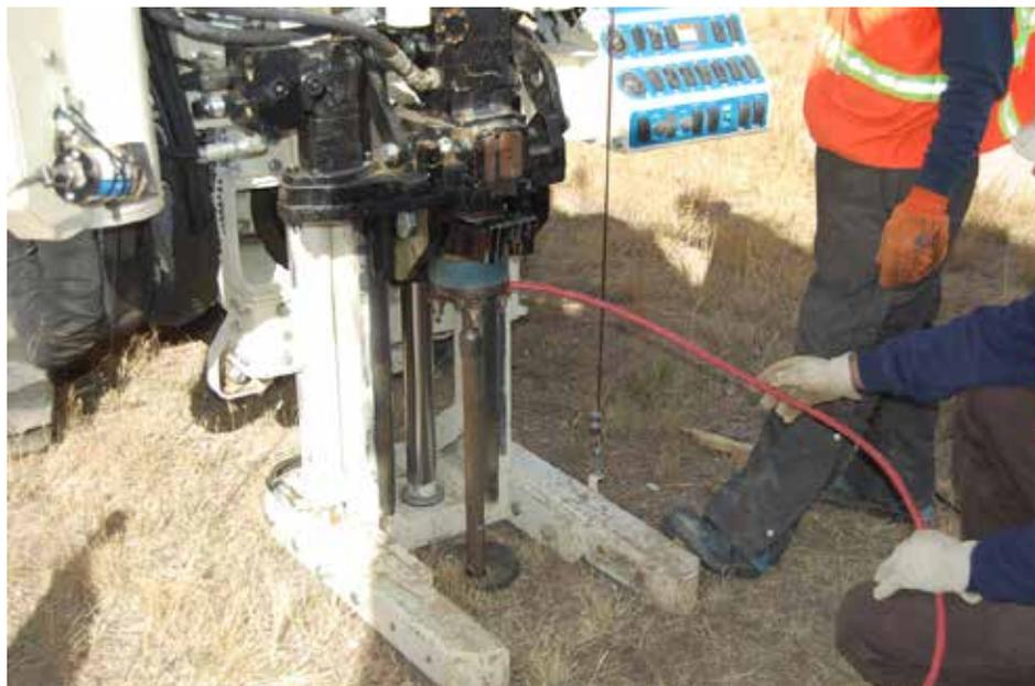
The red tubing shown is what contains the carrier gas that flows between the membrane and the truck mounted field detectors, along with the soil conductivity sensors. The tip of the MIP is designed to fit into any standard direct push rig. The plot of the collected data from a direct push insertion next to MW-173 is reported as Figure 1:
