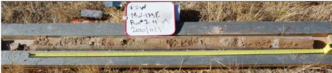
Using this core, a small cylindrical sample of soil is removed by a clean stainless steel cylinder and inserted into a sealed vial containing a known amount of methanol to avoid volatilization losses. This is done at any number of desired depths within the cores. A picture of this process is shown:
