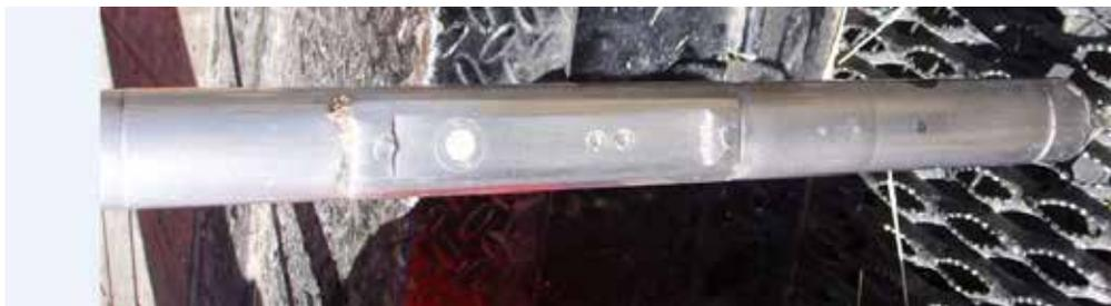
These volatilized VOC's transfer through this membrane, where a carrier gas transfers the VOC's up the tubing and into the truck mounted detectors, such as the FID, ECD or PID. The tip also has the ability to simultaneously measure the soil conductivity, which is plotted alongside the VOC measurements. The MIP process is great for quickly identifying high concentration VOC source zones, in multiple areas on-site.
