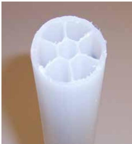
This allows the user of the Multi-Level Sampler to sample from 7 different depth intervals within the groundwater system. This was done in all three monitoring well locations 173, 700 and 38. A picture of a MLS under construction is displayed below:
