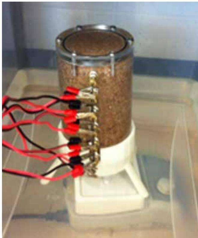
Figure C6-16: DEC in reservoir containing tracer-spiked water.
