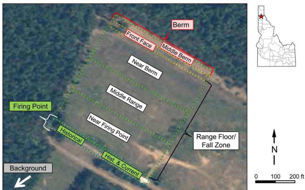
Figure 6.5. Air photo of the Farragut firing range, with overlays showing the boundaries of the decision units. Inset shows the general location of Farragut (from Techlaw 2010).
