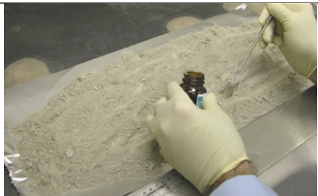
b. At least 30 increments of soil from random locations through the thickness of the sample are combined to form a 10-g subsample.
