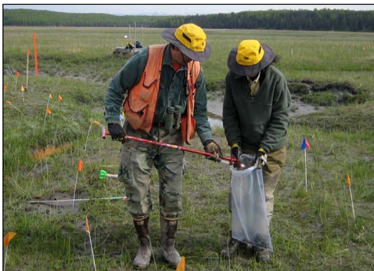
Figure 7.5. Two-person team collecting a multi-increment sample.
