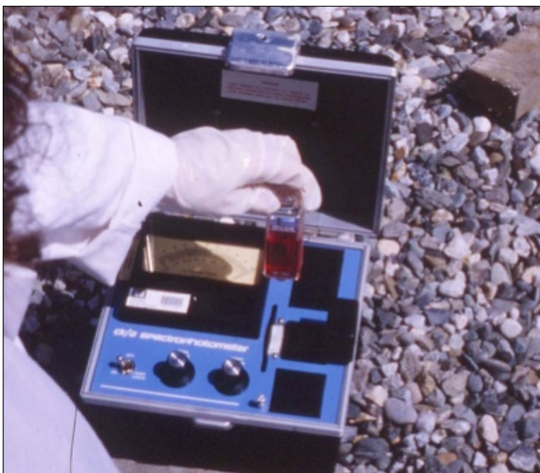
Figure D.3. Portable spectrophotometer used in field to measure concentrations.
