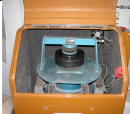
b. LabTech Essa LM-2 Ring Mill
