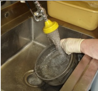
b. Remove gasket from grinder bowl lid and wash all items in soapy water.
