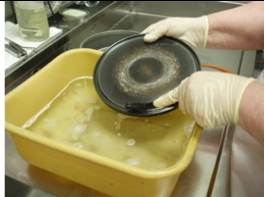
c. Remove adhered soil from the lid, bowl and puck using a brush and scrubbing pad.
