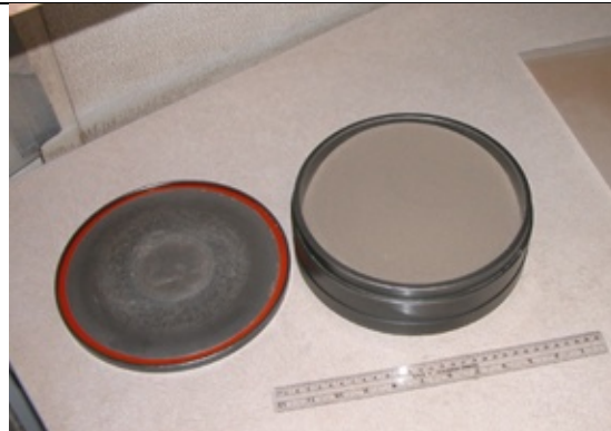
b. LabTech Essa LM-2 Ring Mill
