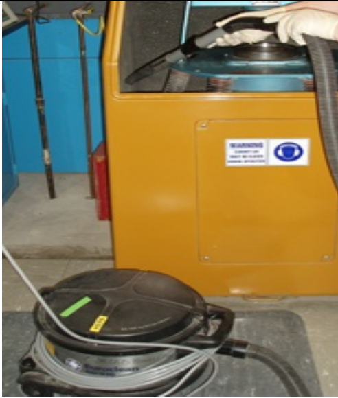
a. Use a HEPA (high efficiency particulate air) vacuum to remove all dust
