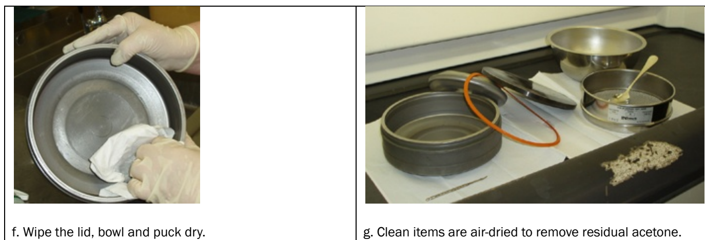
Figure 8.2 How to process a soil sample.
