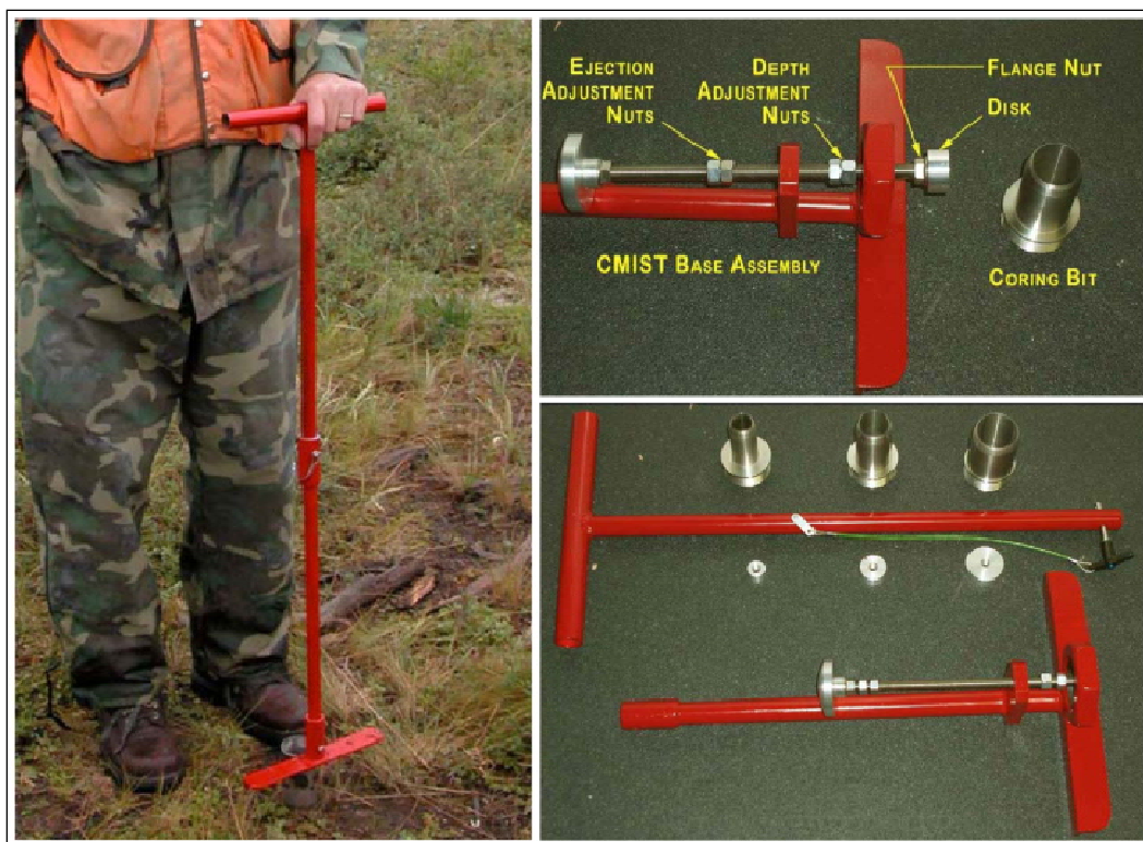
Figure 7.1. CRREL coring device (Walsh M.R. 2009). Note various size coring shoes. Increment cores from a single decision unit should be of the same size
