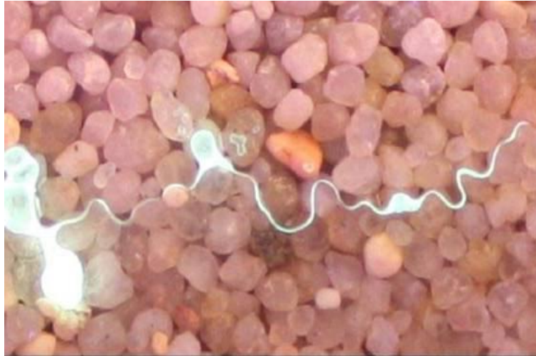
Figure 3. LNAPL moving as an intermediate wetting fluid at the air-water interface in coarse sand (Photo courtesy of Dr. Julio Zimbron).
