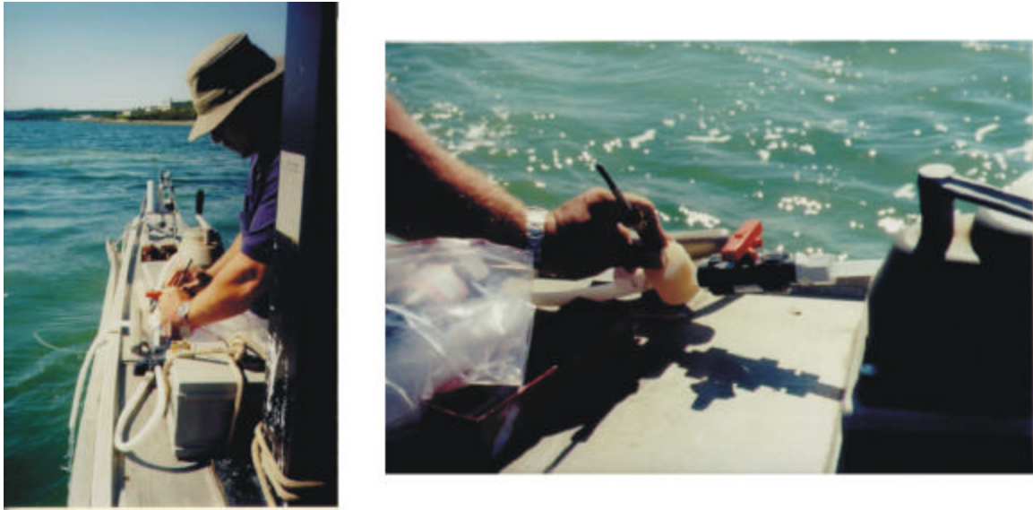
Figure 10. Flow through SPME sampling system being used to collect samples.
