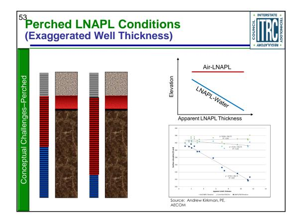
What happens when the LNAPL is sitting on a low-permeability layer? This is often called a perched condition. In this instance, the LNAPL has enough head to continue to migrate downward, but it can't, because it is blocked by the soil pore resistance of the fine-grained layer. The well becomes a pathway for drainage of the LNAPL, so it flows into the well. As the water level in the well drops, more LNAPL can flow in, even though the Air-LNAPL interface stays relatively stationary.
