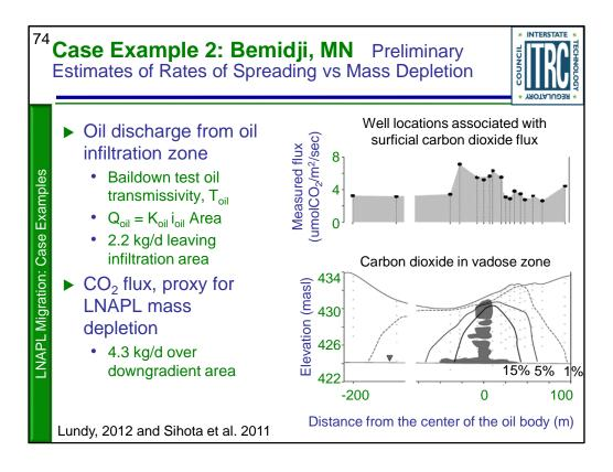
Here are the mass discharge rates...we have 2.2 kg/d of oil phase leaving the infiltration area, and 4.3 kg/d discharging to the atmosphere downgradient of that area.
