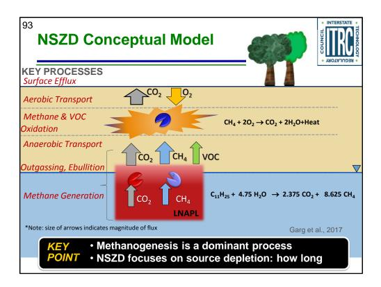
Methane is generated by anaerobic degradation. Methane migrates upward and is aerobically oxidized. The methane oxidation zone can be near the water table, or higher, depending on the rate of CH4 and VOC production, and also if there are shallow soil impacts.
