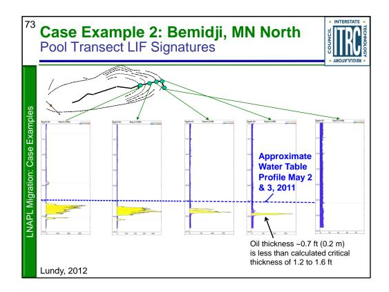
The smaller thickness recorded by the LIF tool is consistent with notion that the oil previously met the critical thickness, but weathering has reduced the thickness.
