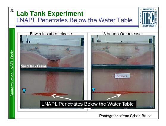
This sand tank experiment shows the release of an LNAPL dyed red. The second image shows that the LNAPL distributes above and below the water table, as expected.
