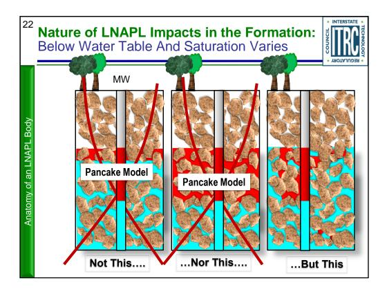
Instead of a layer of continuous uniform LNAPL saturation, LNAPL and water **both exist in the same soil**, in varying amounts. Let's look at this in more detail...
