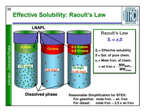
Imagine three LNAPLs: one pure Xylene, one pure Octane, and one that is a mixture of the two. Each closed beaker has LNAPL in equilibrium with water.
