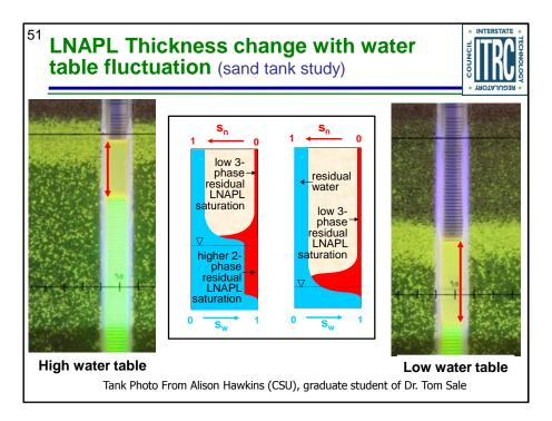
As the water table rises, water displaces LNAPL and air and traps LNAPL in pores.
