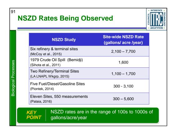
Measured rates, based on CO2 emissions, are <u>much</u> higher than expected based on dissolved phase fluxes alone. What is happening here?
