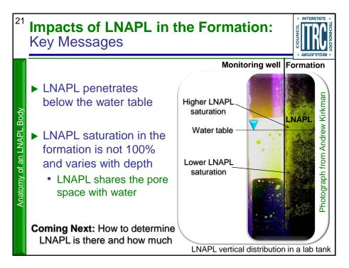
The key message here is that LNAPL doesn't float like a pancake on top of the water table, it penetrates below the water table in a variable saturation profile. This varying saturation arises because the LNAPL and water occupy the same pore space.
