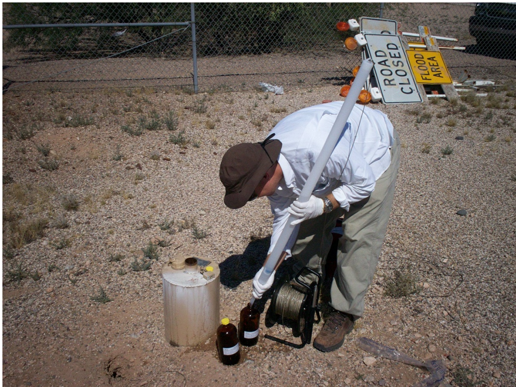
Figure 4. Sample bottles being filled by U.S. Geological Survey employee with groundwater sample taken from a former supply well by a polyethylene bailer.
