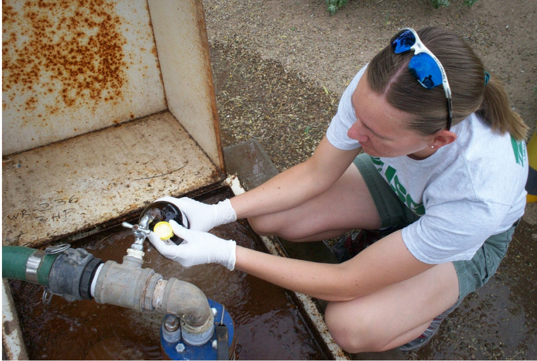
Figure 3. Groundwater sample being collected at monitoring-well head by U.S. Geological Survey employee.
