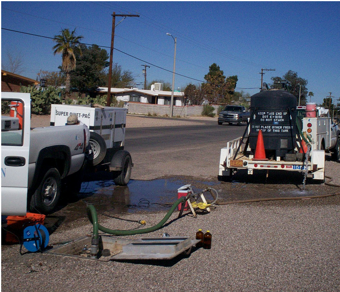
Figure 2. Purging of a TARP-area monitoring well by City of Tucson Water Department personnel prior to groundwater sample collection.
