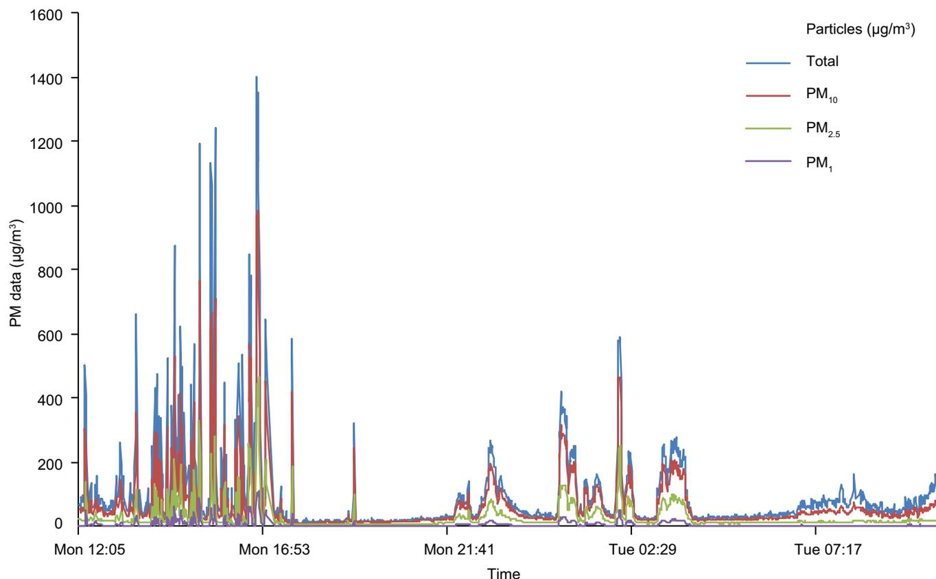
Figure 2: Particulate concentrations from 1 July 2013 to 2 July 2013 at monitoring site 1
