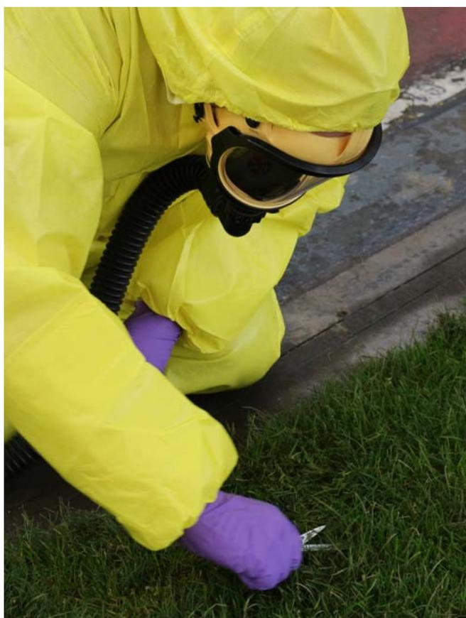
**Figure 1: GDS framework supplier sampling contaminated area (K Halls © Crown copyright 2013 GDS)**
