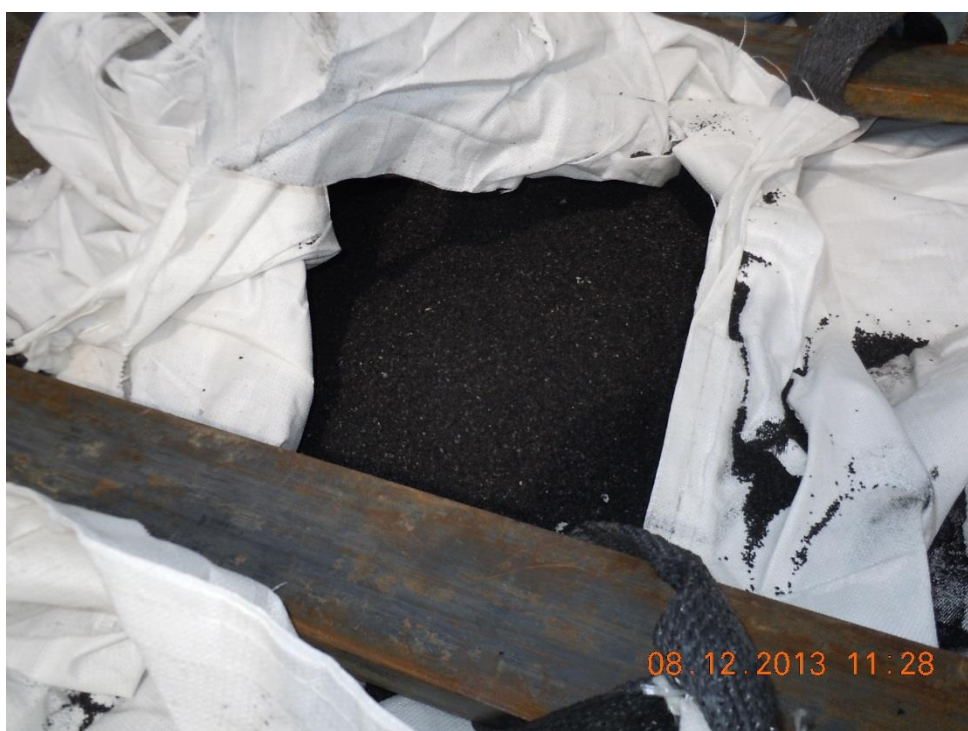
Figure 8.3: Granular activated carbon
