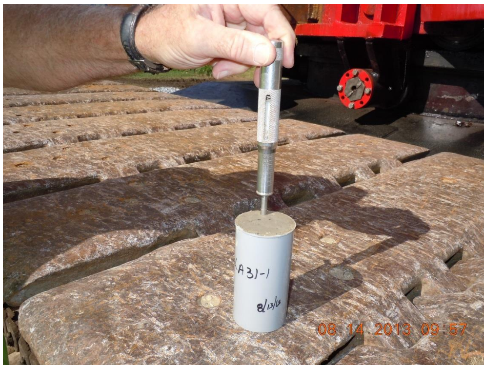
Figure 6.10: Checking set/strength by a pocket penetrometer
