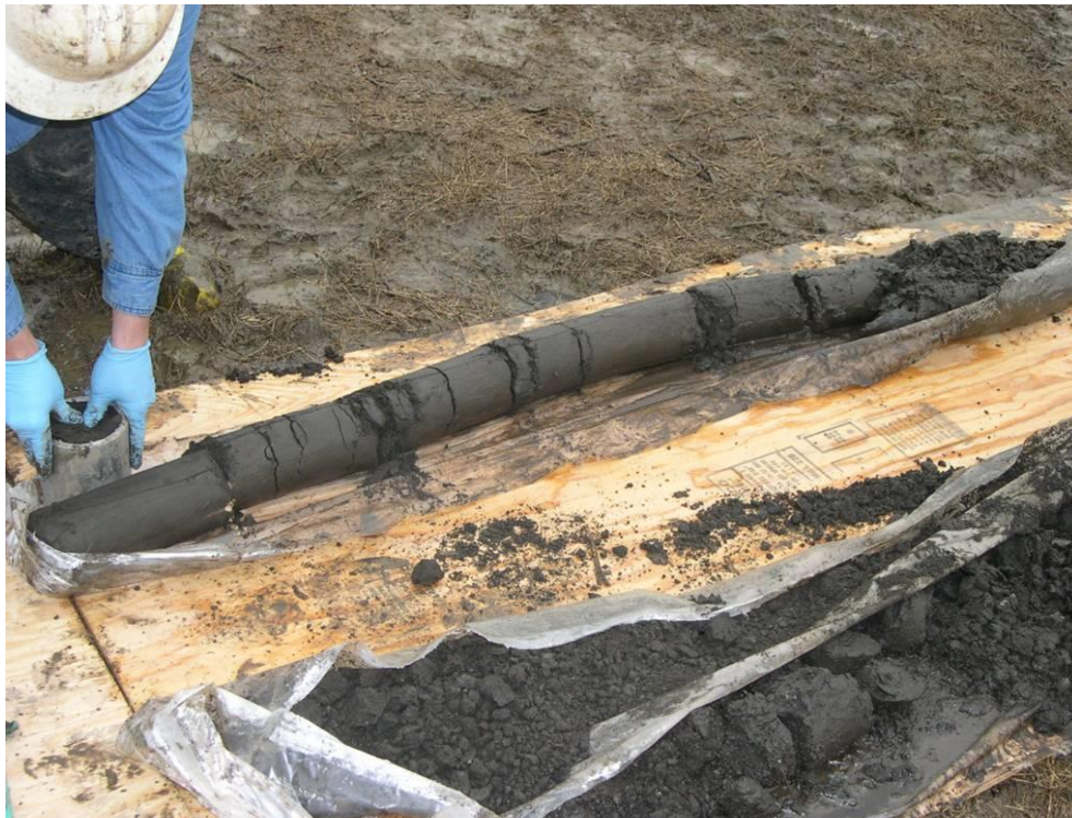
Figure 6.18: Cores obtained by sonic drilling of S/S material
