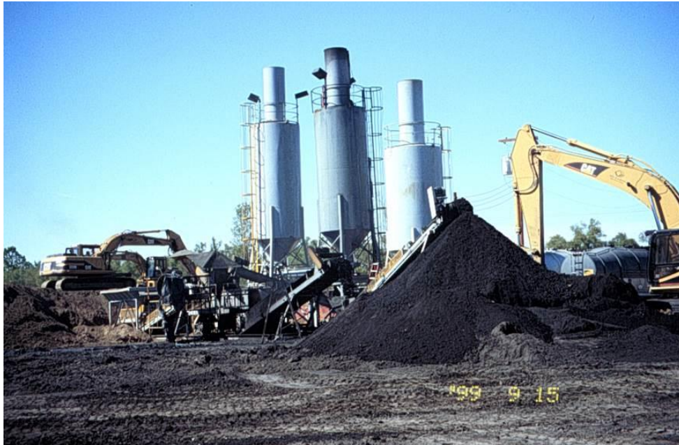
Figure 1.1: Treating creosote, PCP, & dioxins in pug-mill
