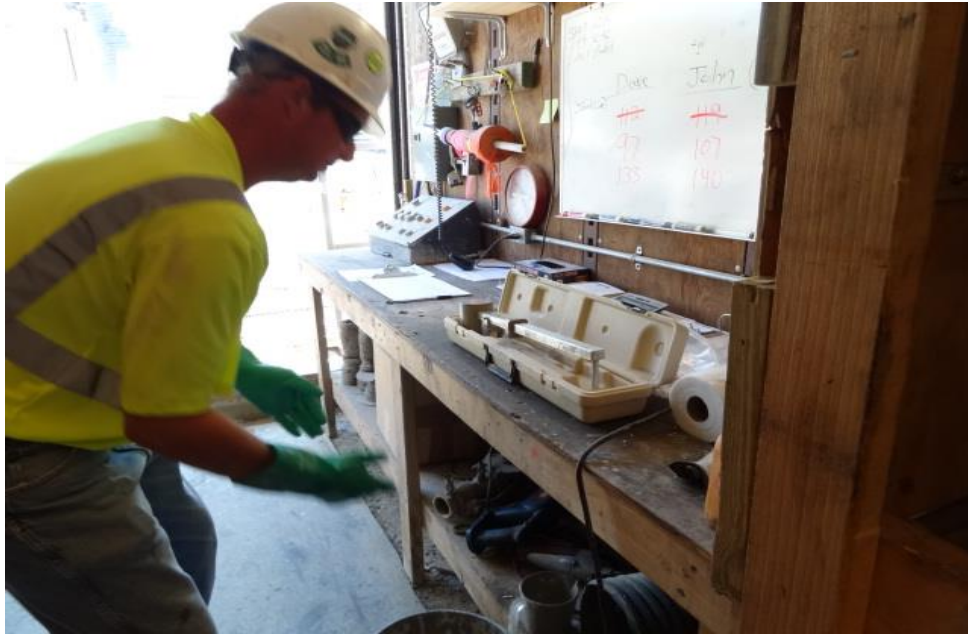
Figure 8.16: Grout density test by mud balance
