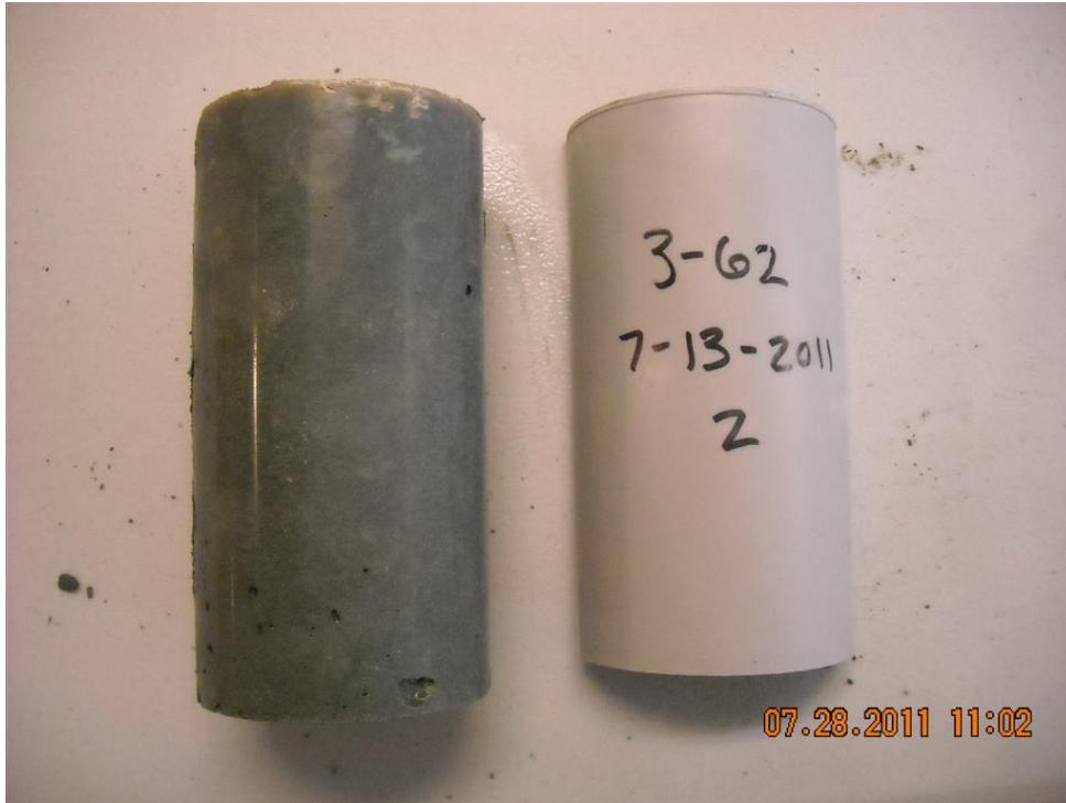
Figure 6.14: A well-prepared specimen with minimal air voids
