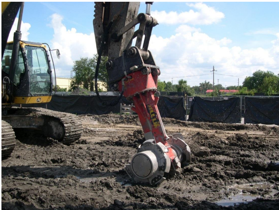
Figure 5.17: Allu mixer head (in red) attached to a standard excavator
