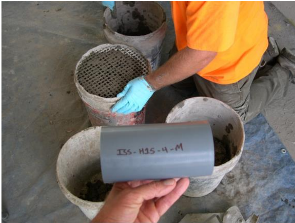
Figure 6.8: Labelling of specimen mold and cap
