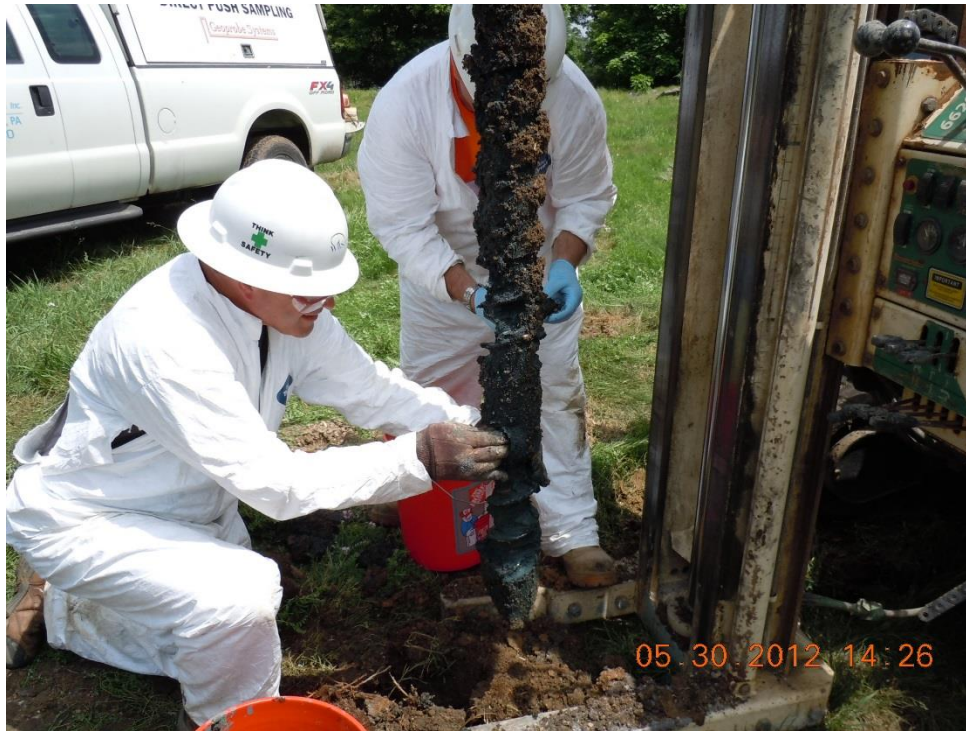
Figure 8.21: Collecting a bulk treatability sample from auger flights
