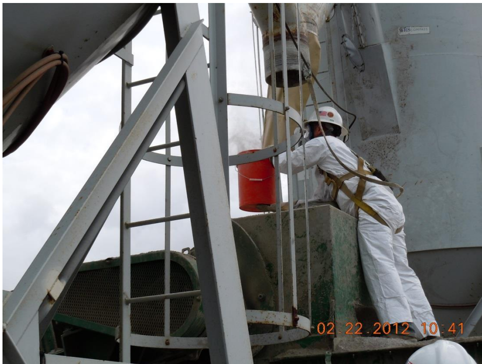
Figure 4.8: Calibrating reagent feed from a screw auger
