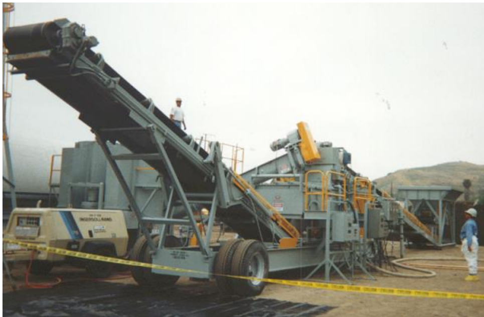
Figure 4.2: A pug-mill with its ancillary equipment
