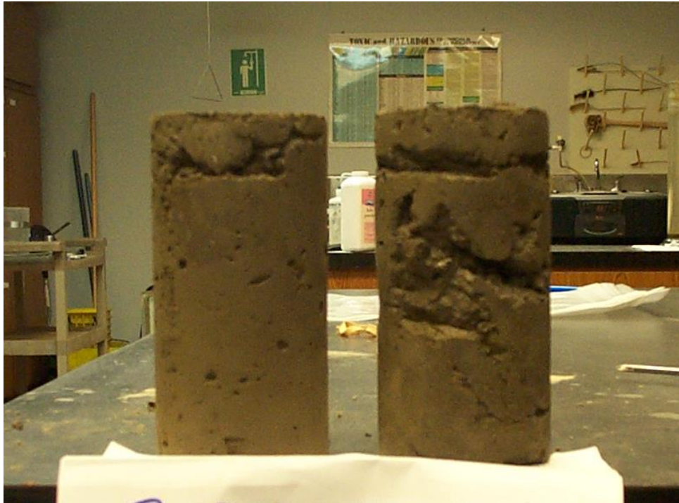
Figure 6.13: Poorly prepared field-specimens
