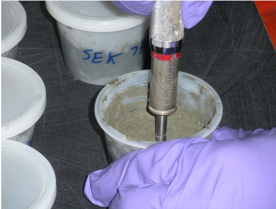
Figure 8.9: Pocket penetrometer testing for approximate strength
