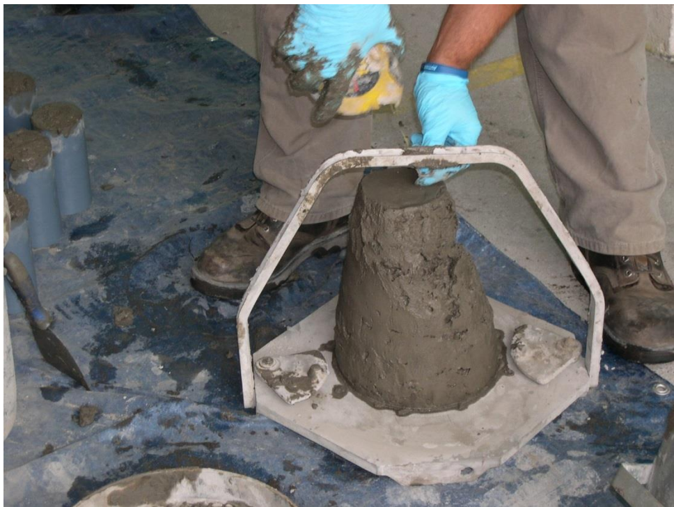
Figure 6.12: A slump test on an S/S bulk sample
