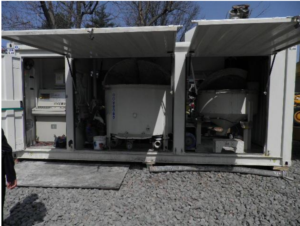
Figure 5.8: An automated batch plant
