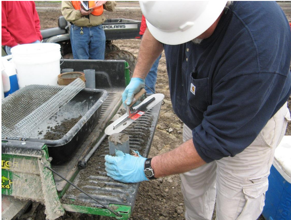
Figure 6.6: Preparing a 3 in x 6 in (75 x 150 mm) mold
