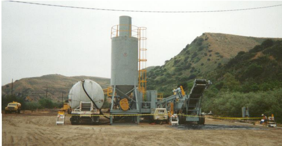
Figure 4.3: Ancillary equipment of a pug-mill
