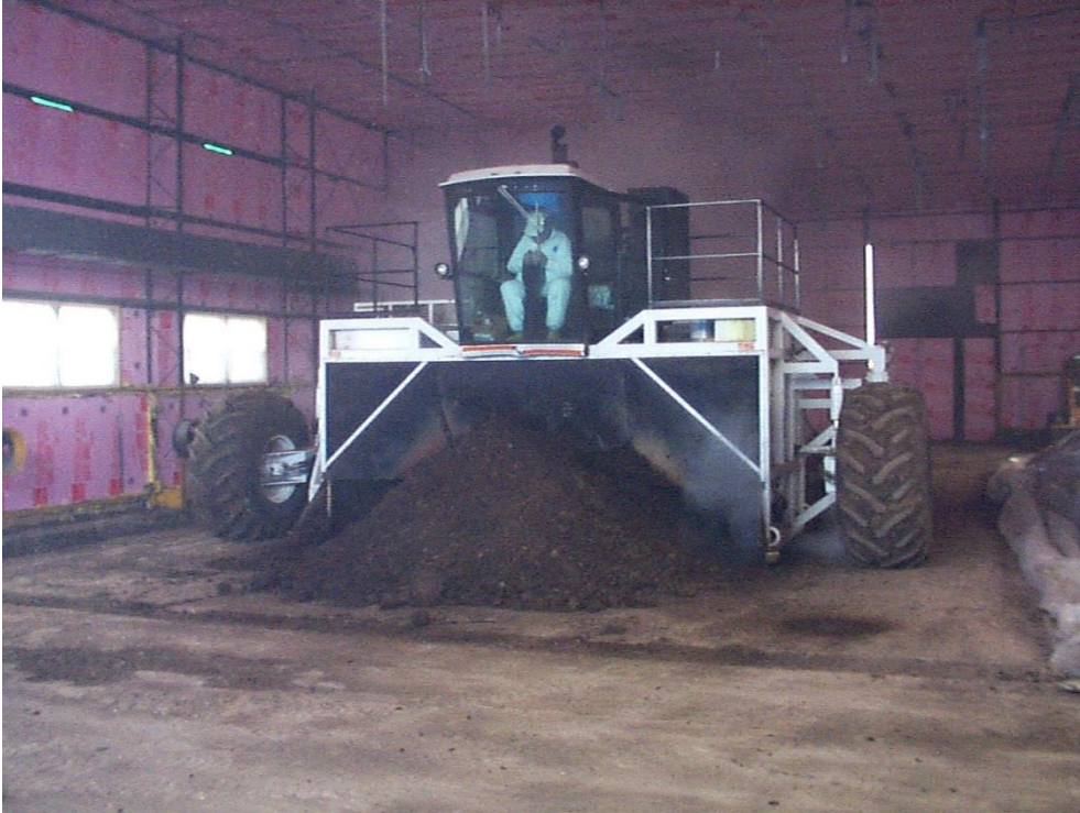
Figure 4.16: Paddle aerator mixing windrowed soil
