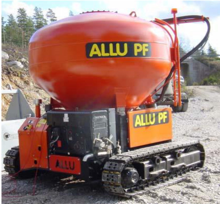
Figure 5.9: Self-propelled dry storage silo
