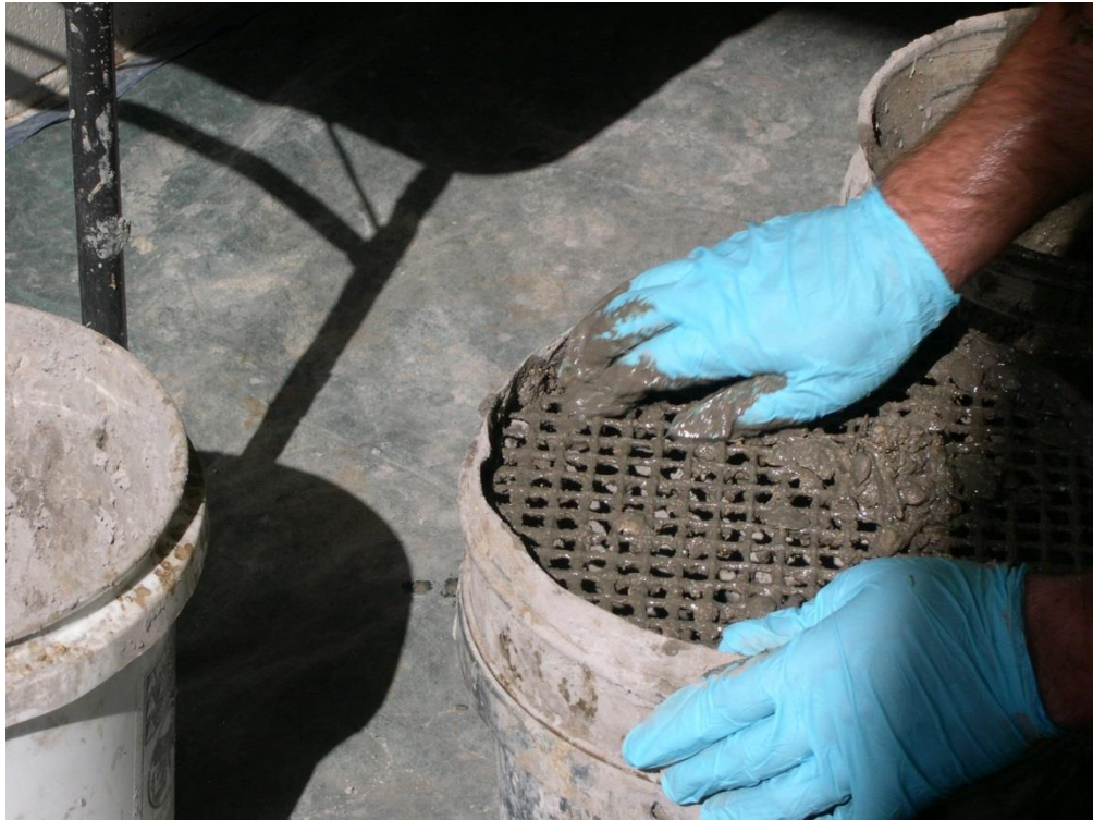
Figure 6.7: A 0.5 in (12.5 mm) screen to remove oversize debris
