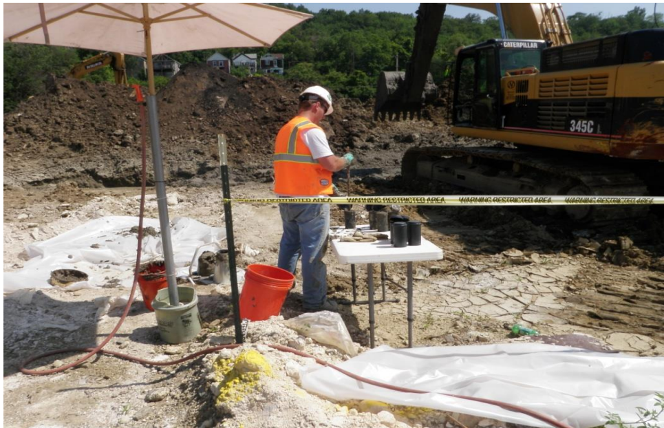
Figure 8.14: Field quality control test specimen preparation
