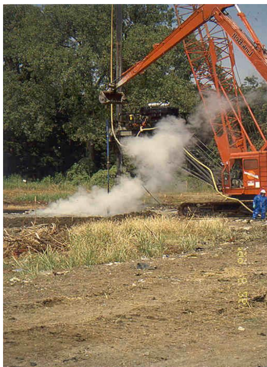
Figure 8.20: In-situ auger test producing steam, sulfur dioxide emissions
