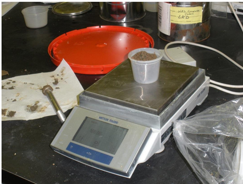
Figure 8.8: Reagents are measured on a weight/weight basis to the untreated soil
