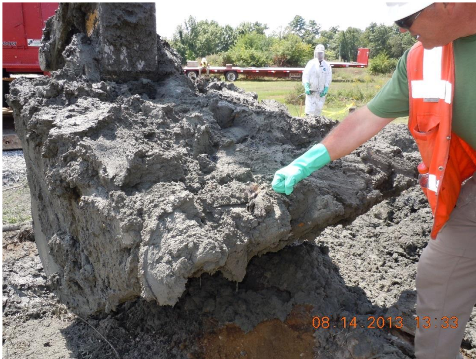
Figure 8.17: Field check to assure homogenous mixing
