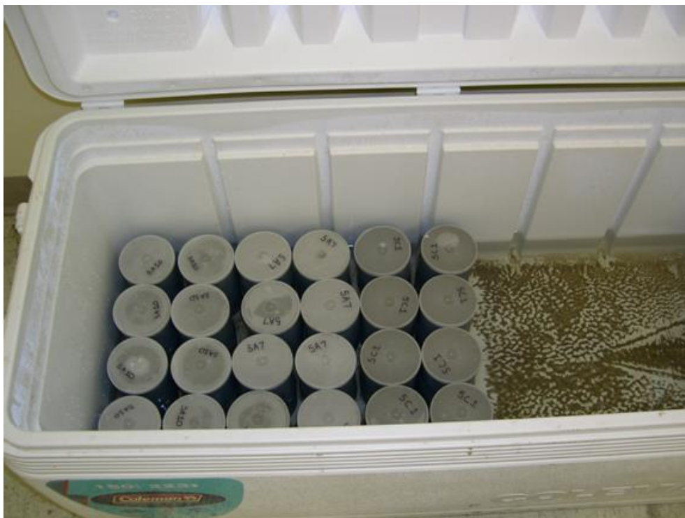
Figure 6.9: Sample molds curing on-site in water bath
