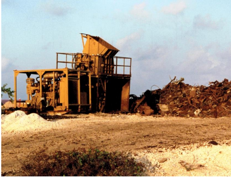
Figure 4.22: A rotary shear shredder processing scrap metal
