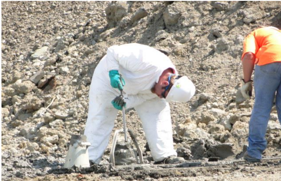
Figure 8.15: Field slump test performance
