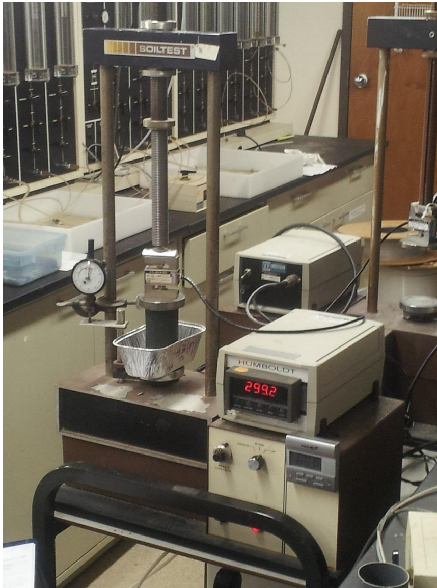
Figure 8.5: Unconfined compressive strength testing
