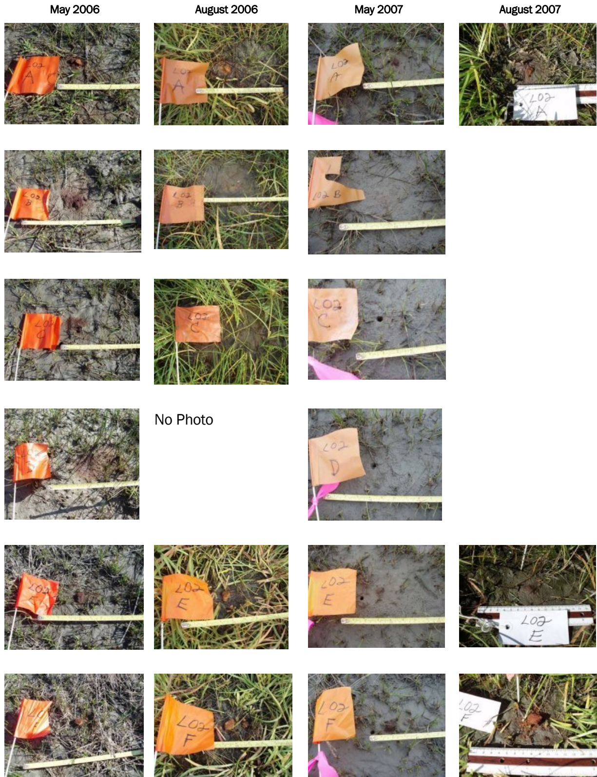
Figure 83. Photos of Comp B chunks dispersed by low-order detonation #2, photographed (l-r) in May and August 2006, and May and August 2007. Missing photographs indicate the loss of HE chunk(s).
