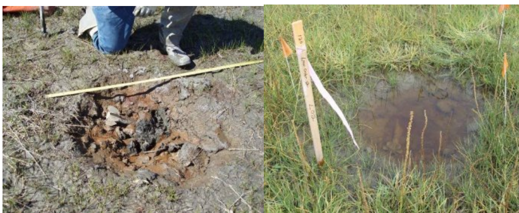
Figure 82. Crater formed by LO 2 detonation at ERF. On the right is the same area after flooding tides and rainfall in August 2006.
