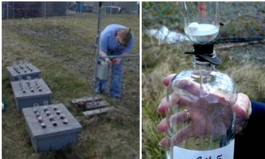
Figure 12. Outdoor tests showing Buchner funnels used to hold the HE pieces. Any precipitation landing in the funnel moved through the glass frit and into 1-L glass bottles in the wooden boxes.
