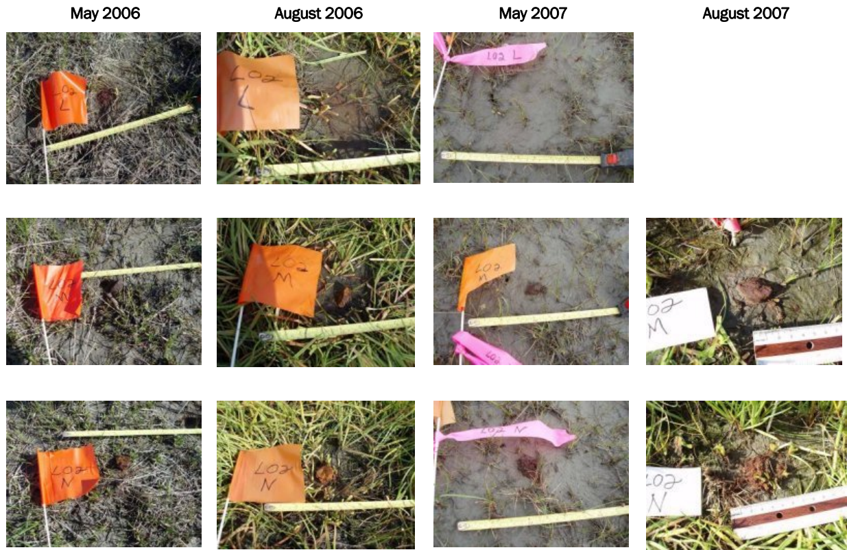
Figure 83 (cont'd). Photos of Comp B chunks dispersed by low-order detonation #2, photographed (l-r) in May 2006, August 2006, May 2007, and August 2007. Missing photographs indicate loss of HE chunk(s).
