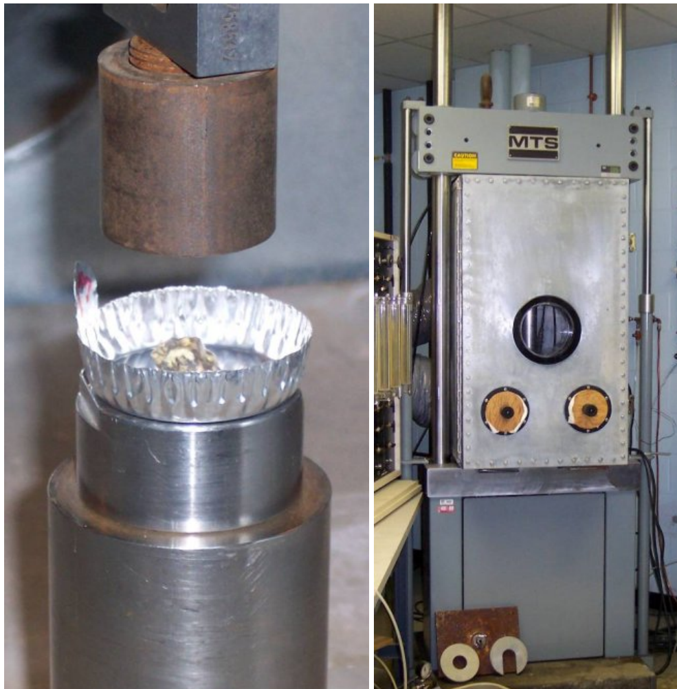
Figure 68. CRREL's Material Testing System (MTS) used to crush explosive particles.
