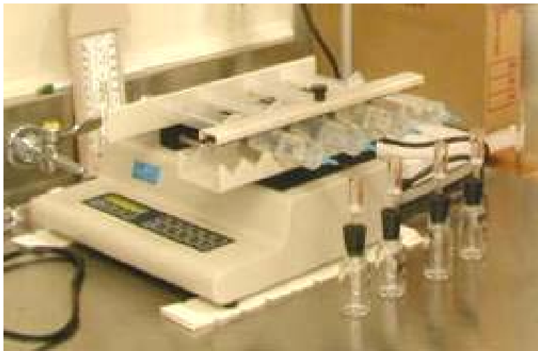
Figure 3. Laboratory setup showing the multiple-syringe pump used to drip water on explosive particles.
