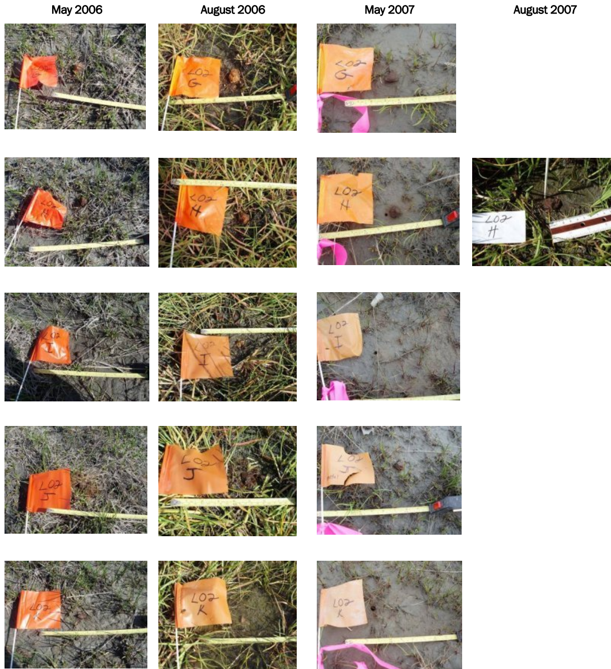
Figure 83 (cont'd). Photos of Comp B chunks dispersed by low-order detonation #2, photographed (l-r) in May and August 2006, and May and August 2007. Missing photographs indicate loss of HE chunk(s).
