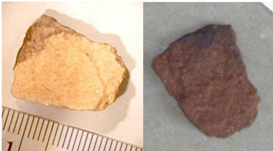
Figure 39. Note the darkening of TNT 4 between when it was set outside on 2 May 2006 (left) and on 30 May 2006 (right).
