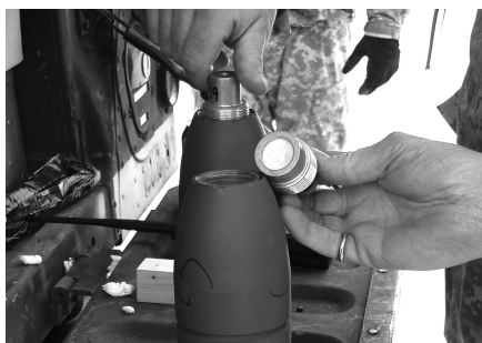
Figure 2. Fuzing for Phase 2 command detonation tests.
