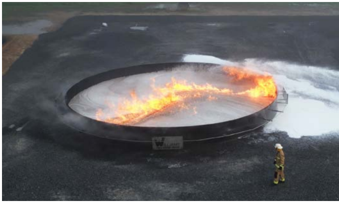
Figure 2. Control achieved on 42-ft tank fire
