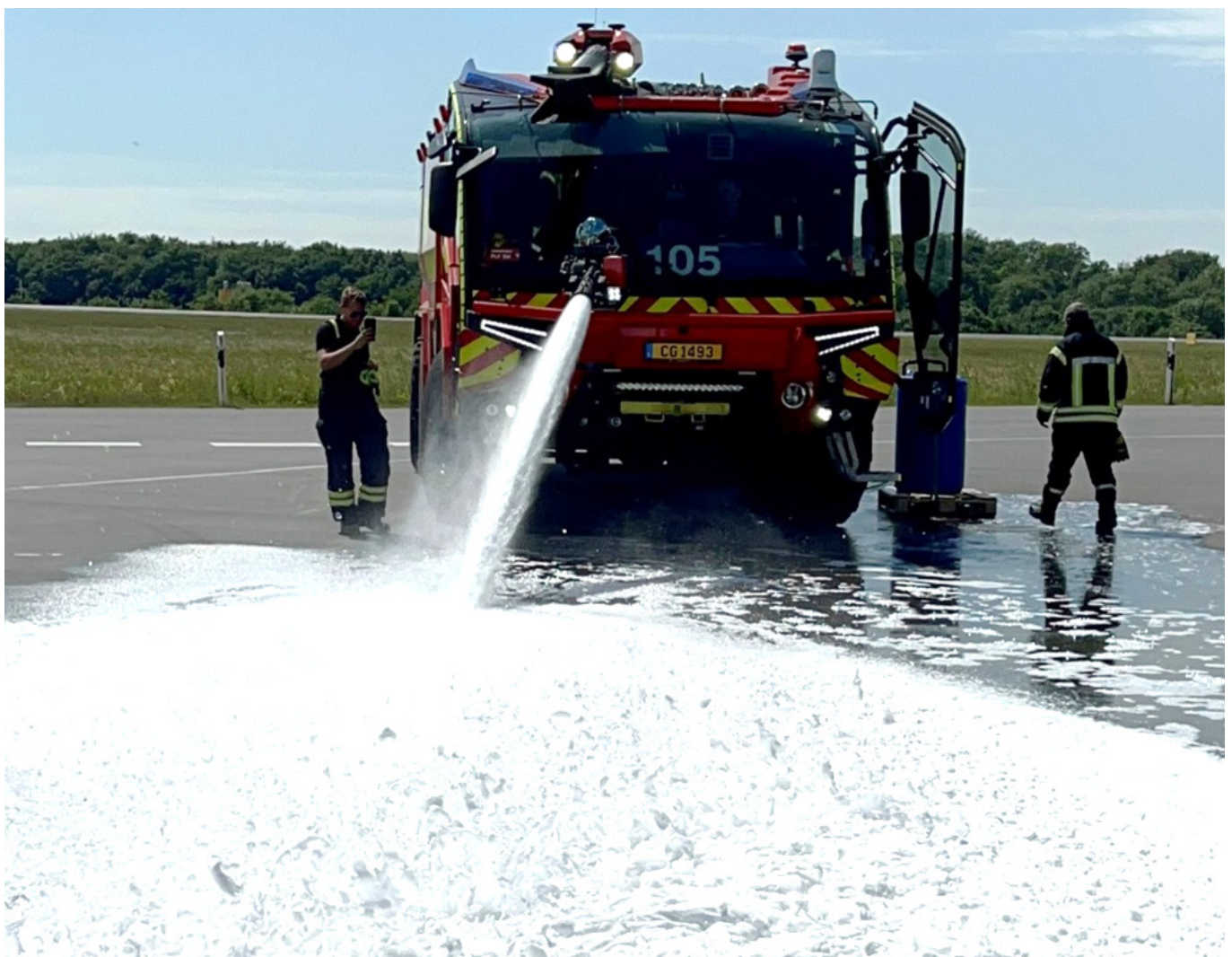
Secondary foam expansion, hitting the pavement through a semi-aspirated nozzle. (Foto: M. Gorski)
