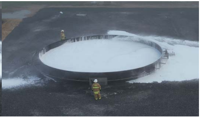
Figure 3. Extinguishment of 42-ft tank fire
