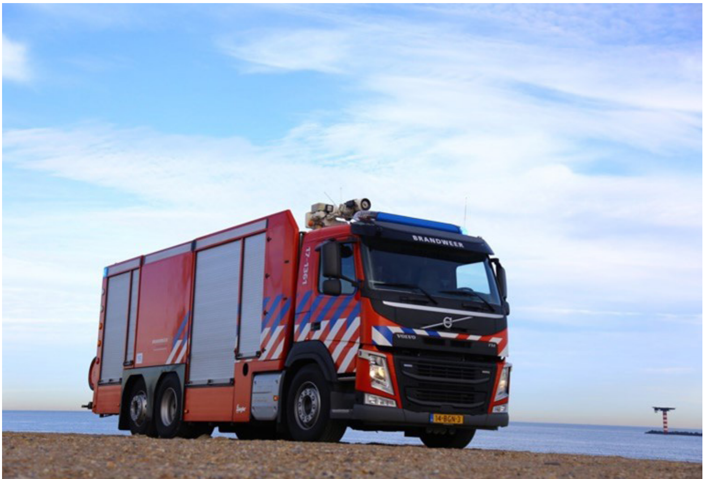
GB's newer industrial foam trucks have 400 l fluorine free foam – Credit: Gezamenlijke Brandweer
