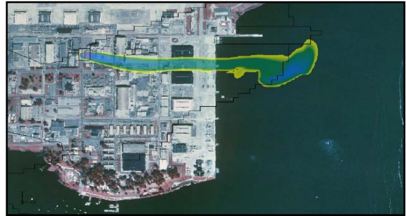
Jacksonville NAS plans to develop ACLs based on a mixing zone analysis
