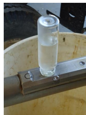
Figure 5.5: 40ml vial of working standard inverted onto membrane
