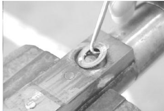
Figure 8.2: Remove and discard the copper washer.
