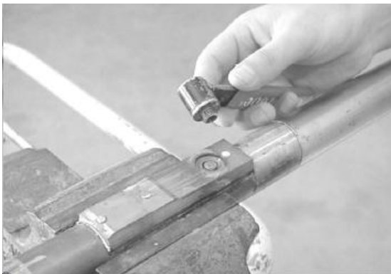
Figure 8.1: Unthread the membrane from the probe block.
