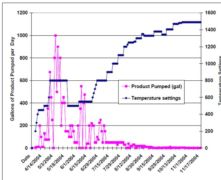
**FIGURE 1. Product recovered as a function of temperature settings (°F) of thermal wells. The first three months comprised the Level 1 phase, after which the temperatures were ramped up to accomplish Level 2/3 heating.**
