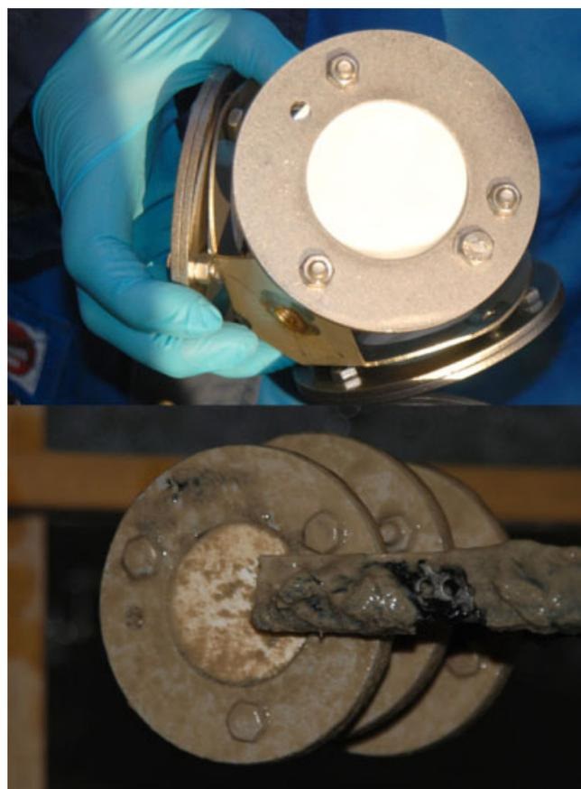
Fig. 1. Differences in polar organic chemical integrative samplers (POCIS) fouling from different deployment environments. Very lightly fouled POCIS (upper picture) deployed in the Norwegian Sea (~200 km offshore) for 42 d and moderately fouled POCIS (bottom picture) from wastewater treatment works after 14 d exposure. [Color figure can be seen in the online version of this article, available at [wileyonlinelibrary.com](http://wileyonlinelibrary.com).]
