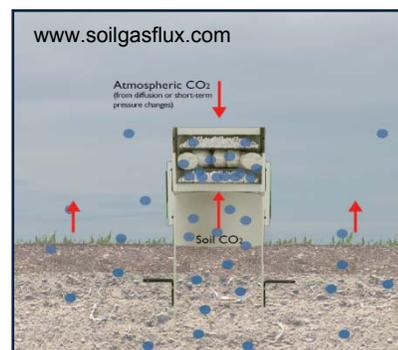
and capture both naturally occurring CO<sub>2</sub> flux from organics in the soil and CO<sub>2</sub> that was generated by hydrocarbon biodegradation. The naturally occurring, background CO<sub>2</sub> signal can be removed from the trap data by analyzing for the carbon 14 isotope and adjusting the measurement of total CO<sub>2</sub> flux (see Frequently Asked Questions in Section 7.5 below; Eflux, 2014; McCoy et al., 2014).
